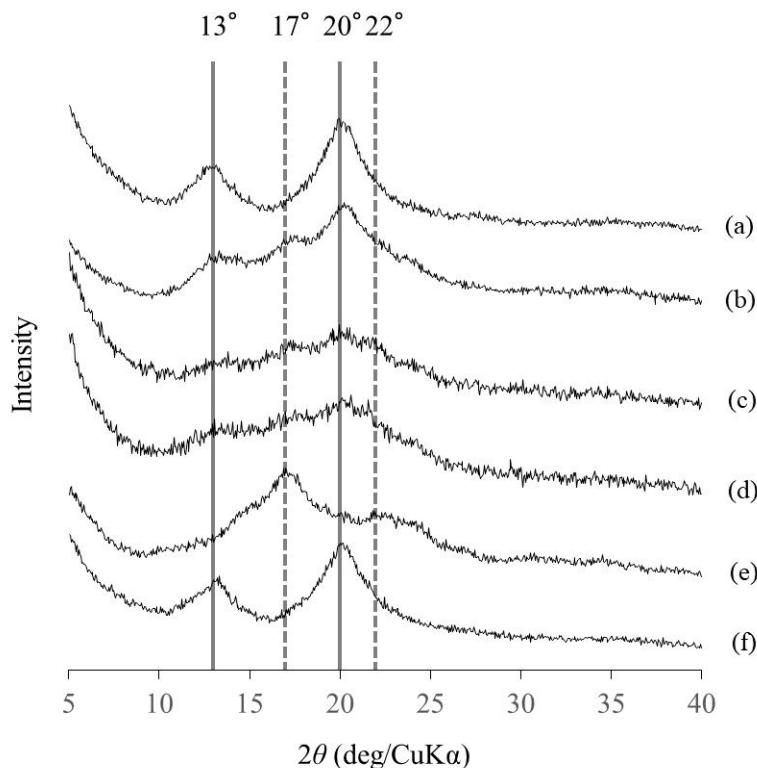
**Figure 2.** X-ray diffraction (XRD) profiles of (a–d) products by lyophilization of runs 1–4, (e) enzymatically synthesized amylose, and (f) amylose-PCL inclusion complex.
