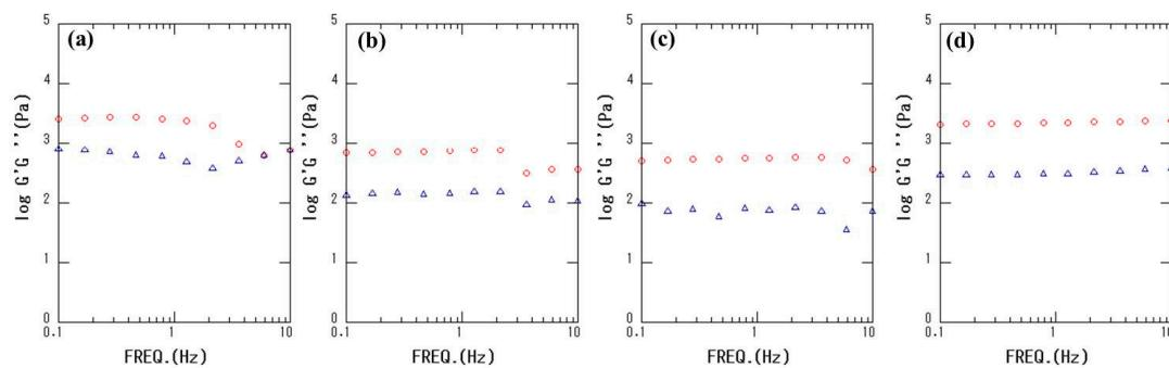
**Figure 4.** Evaluation of storage modulus  $G'$  (circles) and loss modulus  $G''$  (triangles) as a function of frequency for products before lyophilization of run 2 with reaction times of (a–d) 0.5, 1, 3, and 5.
