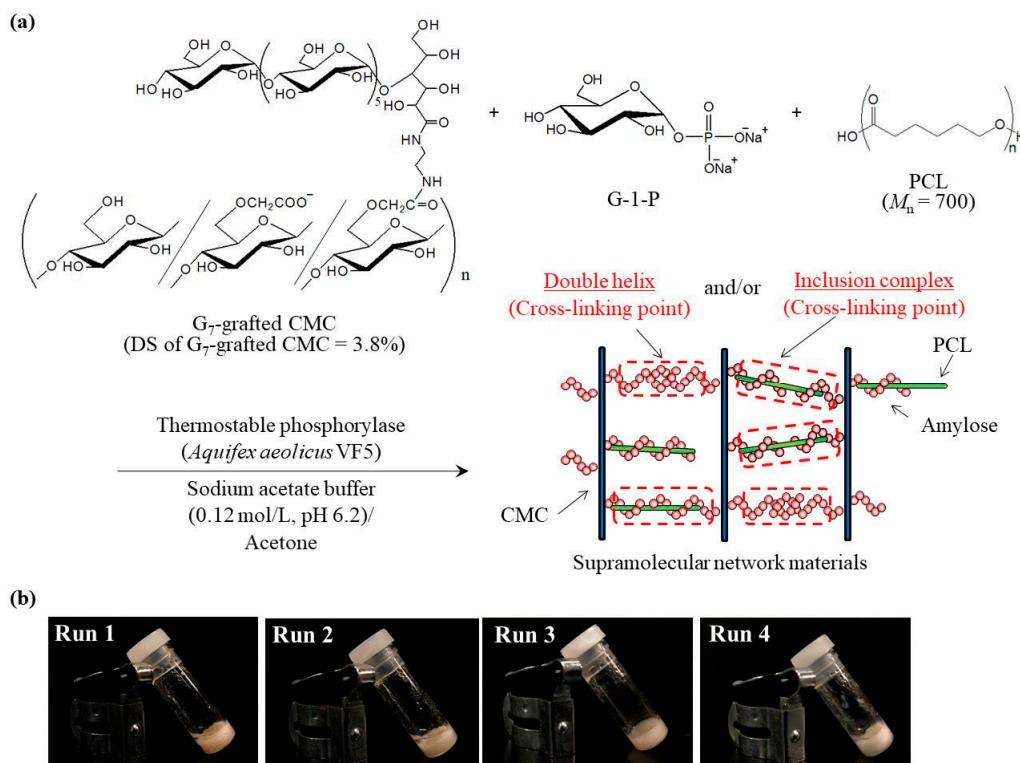
**Figure 1.** (a) Image for preparation of supramolecular network materials by means of amylose helical assemblies formed in phosphorylase-catalyzed enzymatic polymerization, and (b) photographs of reaction mixtures.
