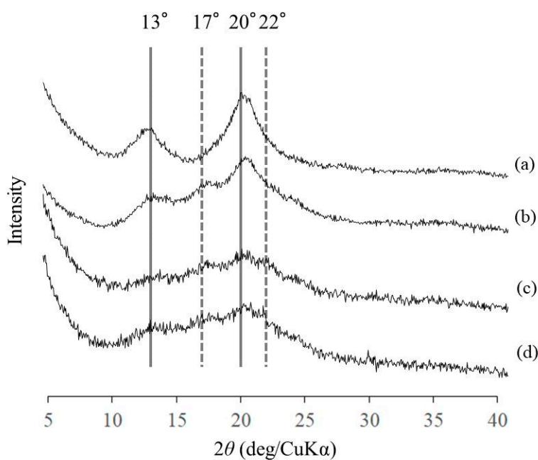
**Figure 3.** XRD profiles of products by lyophilization of run 2 with reaction times of (a–d) 0.5, 1, 3, and 5.
