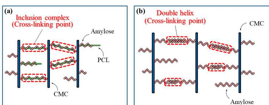
**Figure 6.** Images for (a) smaller and (b) larger network structures cross-linked by inclusion complexes and double helices, respectively.
