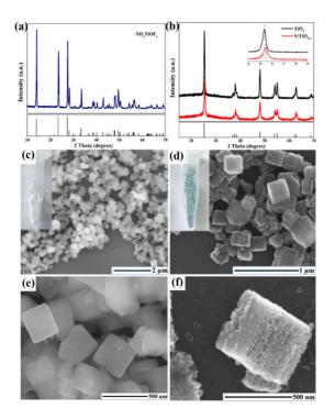
**Figure 19.** Schematic representation of the synthesis of  $TiO_x$  nanosheets. X-ray powder diffraction (XRD) pattern of (a) NH<sub>4</sub>TiOF<sub>3</sub> and (b) N/TiO<sub>2-x</sub>. SEM images of (c,e) NH<sub>4</sub>TiOF<sub>3</sub> and (d,f) N/TiO<sub>2-x</sub> [108]. Copyright 2019 The Royal Society of Chemistry.
