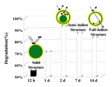
**Figure 16.** Comparison of photocatalytic activities of titania spheres with solid, sphere-in-sphere, and hollow structures [95]. Copyright 2007 American Chemical Society.
