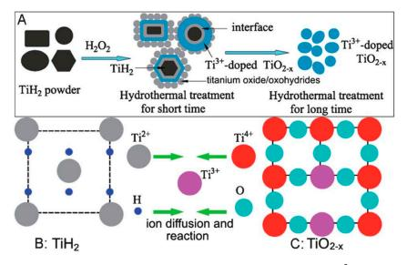
**Figure 8.** (A) Schematic of the formation mechanisms for the rice-shaped  $\text{Ti}^{3+}$  self-doped  $\text{Ti}O_{2-x}$  nanoparticles. (**B**,**C**) The interface diffusion–redox diagram. The green arrows indicate ion diffusion [62]. Copyrighted 2014 The Royal Society of Chemistry.
