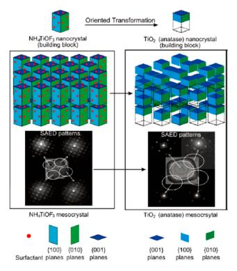
**Figure 17.** Illustration of the oriented transformation of NH<sub>4</sub>TiOF<sub>3</sub> mesophyte to TiO<sub>2</sub> (anatase) mesocrystal [71]. Copyright 2008 American Chemical Society.
