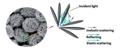
**Figure 15.** Schematic diagram of the reflecting and scattering effects in hierarchical microspheres [94]. Copyright 2014 The Royal Society of Chemistry.
