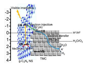
**Figure 18.** Representative scheme of electron injection and movement in g-C3N4 NS (31 wt %)/TMC during visible-light irradiation [106]. Copyright 2017 American Chemical Society.
