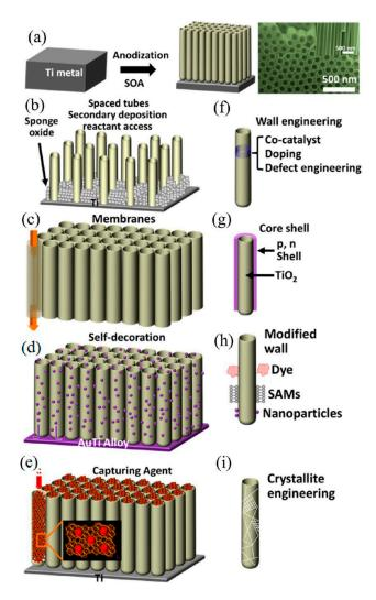
**Figure 13.** Schematic drawing of (a,b) formation and (c-i) modification of anodic nanotube arrays (as discussed in the text) [82]. Copyright 2017 American Chemical Society.
