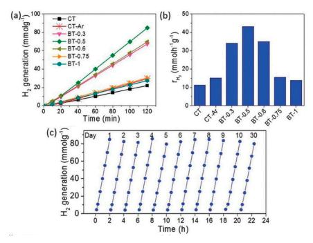
**Figure 10.** (a) H<sub>2</sub> generation profile, (b) rate (rH<sub>2</sub>) of hydrogen generation for different samples, and (c) the stability study of the sample BT-0.5 under the full solar wavelength range of light [70]. Copyright 2015 The Royal Society of Chemistry.
