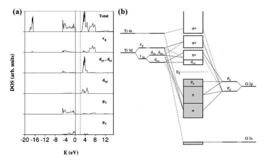
**Figure 2.** (a) Total and projected densities of states (DOS) of the anatase  $TiO_2$  structure and (b) molecular orbital bonding structure for anatase  $TiO_2$  [18]. Copyright 2004 The American Physical Society.
