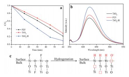
**Figure 21.** Photocatalytic decomposition of MB (**a**) and •OH generation measurement (**b**) of TiO<sub>2</sub> and TiO<sub>2</sub>–H under UV–Vis light irradiation. Schematic illustration (**c**) of the hydrogenation effect on the structural change in TiO<sub>2</sub> and TiO<sub>2</sub>–H [114]. Copyright 2012 The Royal Society of Chemistry.
