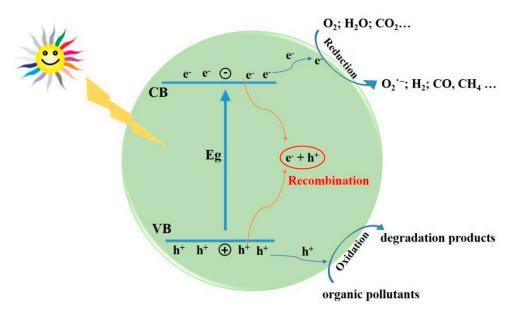
Figure 1. Photocatalytic process in semiconductor.
