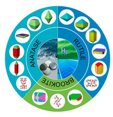
**Figure 14.** Summary of main shapes and applications (i.e., lithium ion batteries, photocatalytic hydrogen evolution, photodegradation, and solar cells) of anatase, rutile, and brookite TiO<sub>2</sub> crystals with their surfaces consisting of different Facets [89]. Copyright 2014 American Chemical Society.
