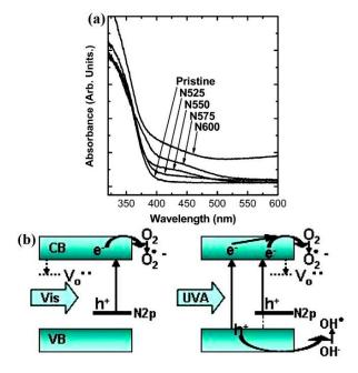
**Figure 7.** (a) Diffuse reflectance spectra of the anatase TiO<sub>2</sub> nanobelts before and after heat treatment in ammonia gas flow at different temperatures and (b) the band structure of N-doped-TiO<sub>2</sub> under visible and UV light irradiation [50]. Copyright © 2009 American Chemical Society.
