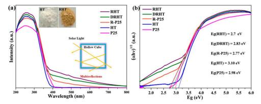
**Figure 11.** (**a**) UV–Vis diffuse reflectance spectra and (**b**) Tauc plot for band gap determination [73]. Copyright 2018 Springer Nature Publishing AG.
