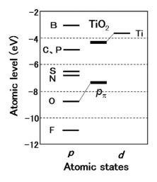
**Figure 6.** Comparison of atomic p levels among anions. The band gap of TiO<sub>2</sub> is formed between the O  $2p\pi$  and Ti 3d states [39]. Copyright 2014 American Chemical Society.
