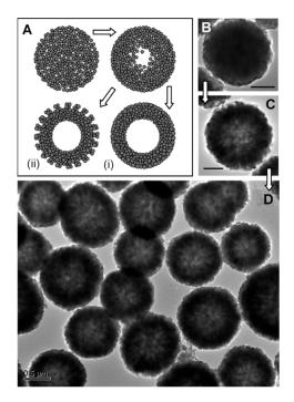
**Figure 12.** (**A**) Schematic illustration (cross-sectional views) of the ripening process and two types (i and ii) of hollow structures. Evolution (TEM images) of TiO<sub>2</sub> nanospheres synthesized with 30 mL of TiF<sub>4</sub> (1.33 mM) at 180 °C with different reaction times: (**B**) 2 h (scale bar = 200 nm), (**C**) 20 h (scale bar = 200 nm), and (**D**) 50 h (scale bar = 500 nm) [75]. Copyright 2004 American Chemical Society.
