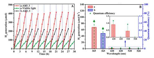
**Figure 22.** Photocatalytic hydrogen evolution of ordered mesoporous black  $TiO_2$  (a) and pristine ordered mesoporous  $TiO_2$  materials (b). (A) Cycling tests of photocatalytic hydrogen generation under AM 1.5 and visible light irradiation. (B) The photocatalytic hydrogen evolution rates under single-wavelength light and the corresponding QE. The inset enlarges the QE of single-wavelength light at 420 and 520 nm [133]. Copyright 2014 American Chemical Society.
