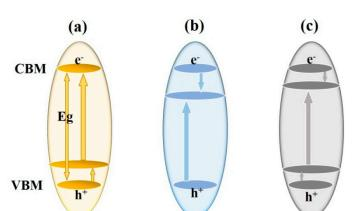
**Figure 3.** Three schemes of the band gap modifications of TiO<sub>2</sub> match the solar spectrum: (**a**) a higher shift in valence band maximum (VBM); (**b**) a lower shift in conduction band minimum (CBM); and (**c**) continuous modification of both VBM and CBM.
