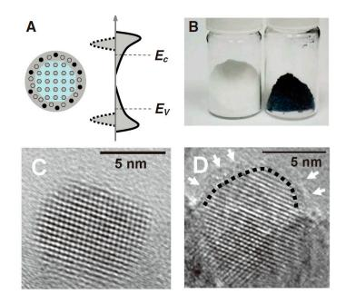
**Figure 9.** (A) Schematic illustration of the structure and electronic DOS of a semiconductor in the form of a disorder-engineered nanocrystal with dopant incorporation. (B) A photo comparing unmodified white and disorder-engineered black  $TiO_2$  nanocrystals. (C,D) HRTEM images of  $TiO_2$  nanocrystals before and after hydrogenation, respectively [54]. Copyright 2011 American Association for the Advancement of Science.
