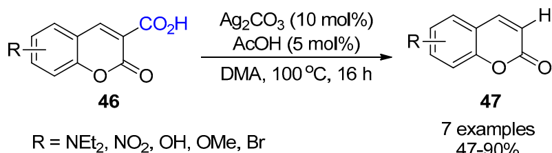
Scheme 30. Ag-catalyzed protodecarboxylation of coumarin-3-carboxylic acid.
