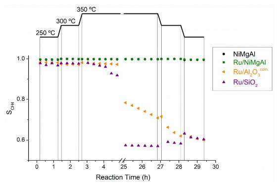
Figure 6. Evolution of CH<sub>4</sub> selectivity with time and temperature during the screening protocol.
