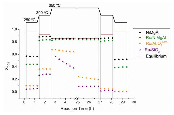
**Figure 5.** Evolution of  $CO_2$  conversion with time and temperature during the screening protocol. Red line shows equilibrium conversion.
