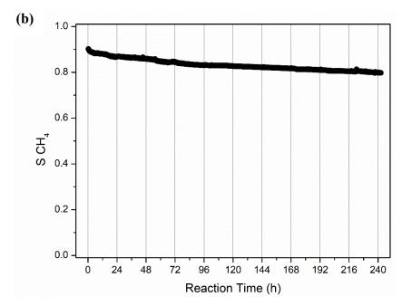
**Figure 7.** (a) CO<sub>2</sub> conversion and (b) CH<sub>4</sub> selectivity obtained with NiMgAl during the long stability test at 350 °C with a weight hourly space velocity (*WHSV*) of 24,000 mL<sub>N,CO2</sub>·g<sup>-1</sup>·h<sup>-1</sup>. Red line shows equilibrium conversion.
