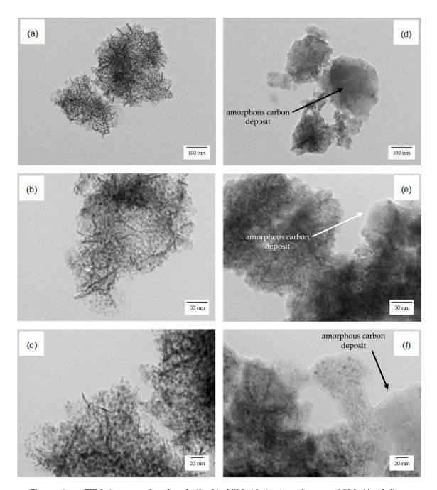
**Figure 8.** TEM images of reduced (fresh) NiMgAl (**a**–**c**) and spent NiMgAl (**d**–**f**) at different magnifications.
