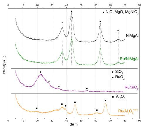
Figure 2. XRD patterns of the catalysts before reduction.
