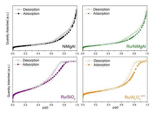
Figure 3. Adsorption/desorption isotherms of nitrogen over all samples.
