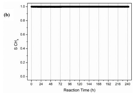
**Figure 10.** (a) CO<sub>2</sub> conversion and (b) CH<sub>4</sub> selectivity obtained with NiMgAl during the long stability test at 300 °C with a WHSV of 2400 mL<sub>N.CO2</sub>·g<sup>-1</sup>·h<sup>-1</sup>. Red line shows equilibrium conversion.
