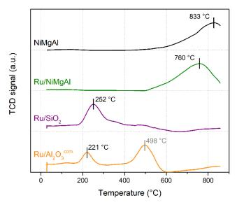
Figure 1. TPR profiles of the tested catalysts.
