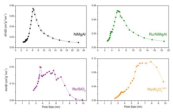
Figure 4. Pore size distribution of the catalysts.
