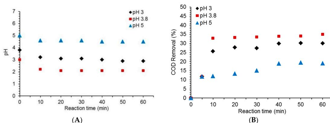
**Figure 1.** The pH profile (A) and removal of chemical oxygen demand (COD) (B) by the Fenton reaction at different pH for the ratio of  $[\text{H}_2\text{O}_2]$  to  $[\text{COD}] = 0.12$  (g/g) and the ratio of  $[\text{H}_2\text{O}_2]$  to  $[\text{Fe}^{3+}] = 50$  (g/g).
