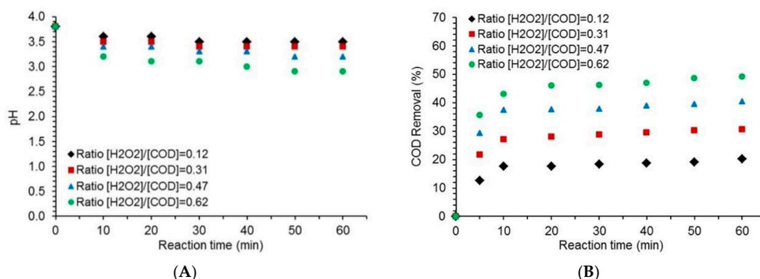
**Figure 2.** The pH profile (A) and removal of COD (B) by the Fenton reaction at different  $[H_2O_2]$  to  $[COD]$  ratios for pH = 3.8 (without adjustment) and the ratio of  $[H_2O_2]$  to  $[Fe^{3+}] = 50$  (g/g).
