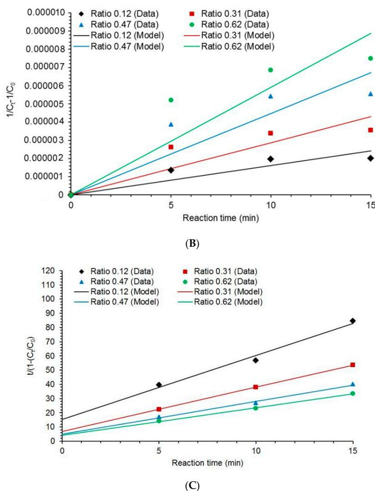
**Figure 5.** Kinetic models for COD degradation at different [H<sub>2</sub>O<sub>2</sub>] to [COD] ratios: (A) first order, (B) second order, and (C) BMG.
