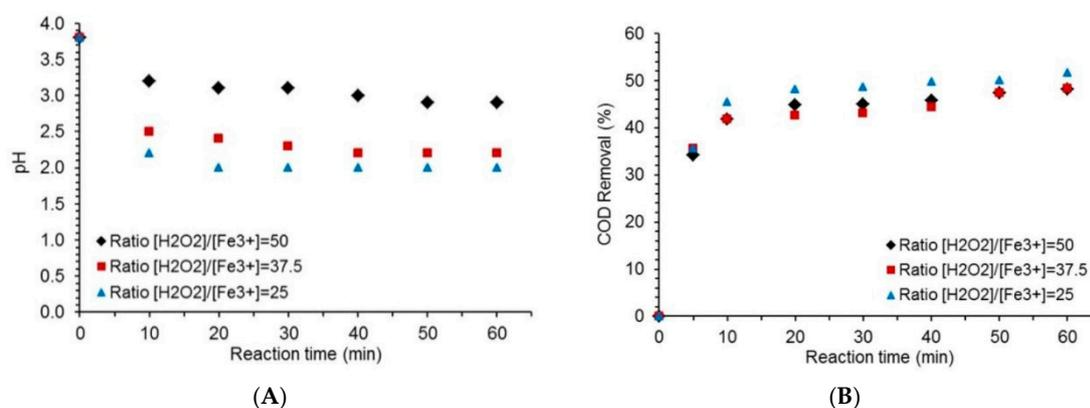
**Figure 3.** The pH profile (A) and removal of COD (B) by the Fenton reaction at different  $[\text{H}_2\text{O}_2]$  to  $[\text{Fe}^{3+}]$  ratios for pH = 3.8 (without adjustment) and the ratio of  $[\text{H}_2\text{O}_2]$  to  $[\text{COD}] = 0.62$  (g/g).
