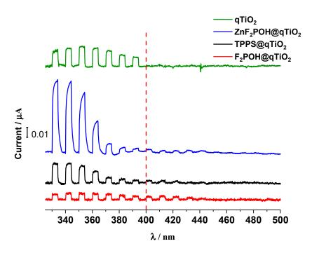
**Figure 6.** The photocurrent measurements as a function of the wavelength of incident light for sulfonated porphyrin (TPPS) and halogenated derivatives  $F_2POH@qTiO_2$ ,  $ZnF_2POH@qTiO_2$  adsorbed at the surface of TiO<sub>2</sub>, as well as bare qTiO<sub>2</sub> as reference at the potential of 1000 mV vs. Ag/AgCl.
