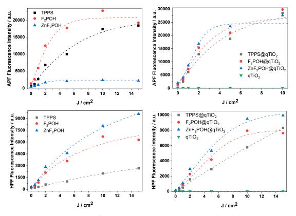
**Figure 7.** Photogeneration of reactive oxygen species (ROS). Light dose-dependent increase of fluorescence of fluorescent probes (10  $\mu$ M): 3-p-(aminophenyl)fluorescein (APF), and 3-p-(hydroxyphenyl)fluorescein (HPF) in the presence of porphyrins and porphyrins at the surface of qTiO<sub>2</sub> materials irradiated with 420 ± 20 nm LED light.
