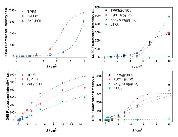
**Figure 8.** Photogeneration of ROS. Light dose-dependent increase of fluorescence of fluorescent probes (10  $\mu$ M): dihydroethidium (DHE), and Singlet Oxygen Sensor Green (SOSG) in the presence of porphyrins and porphyrin-modified qTiO<sub>2</sub> materials irradiated with 420 ± 20 nm LED light.
