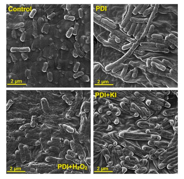
**Figure 10.** SEM images of *Escherichia coli* before PDI treatment (control) and bacterial cell debris after different PDI procedures (2 h incubation, 10 J/cm<sup>2</sup>, 420  $\pm$  20 nm LED light, material concentration of 0.5 g/L with addition of 100 mM H<sub>2</sub>O<sub>2</sub> or 100 mM KI).
