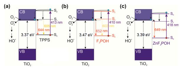
**Figure 5.** Proposed mechanism of the TiO<sub>2</sub> photosensitization, fluorescence emission, and possible pathway of hydroxyl radical generation after excitation of (**a**) TPPS@qTiO<sub>2</sub>, (**b**) F<sub>2</sub>POH@qTiO<sub>2</sub>, and (**c**) ZnF<sub>2</sub>POH@qTiO<sub>2</sub>. CB—conduction band; VB—valence band.
