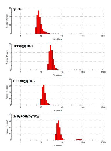
Figure 2. Size distribution of nanocrystalline materials in the aqueous solution.
