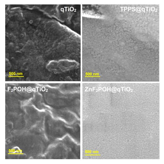
**Figure 3.** SEM images of nanostructured qTiO<sub>2</sub>, TPPS@qTiO<sub>2</sub>, F<sub>2</sub>POH@qTiO<sub>2</sub>, and ZnF<sub>2</sub>POH@TiO<sub>2</sub> recorded on carbon tape.
