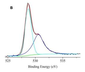
**Figure S5B.** Al K $\alpha$  excited XPS of the Ru/CeO<sub>2</sub> in the O 1s energy region. The black line refers to the experimental profile; the green line refers to the background; the cyan line refers to the 528.7 eV peak; the blue line refers to the 530.6 eV peak; the red line, superimposed to the experimental profile, refers to the sum of the Gaussian components.
