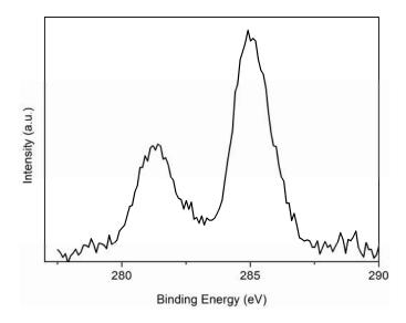
**Figure S3.** Al K $\alpha$  excited XPS of the 1%Ru/CeO<sub>2</sub> in the Ru 3d – C 1s energy region. The peak at 281.3 eV is due to the Ru 3d<sub>5/2</sub> state, the peak at 285.0 eV is due both to the adventious carbon and Ru 3d<sub>3/2</sub> state.
