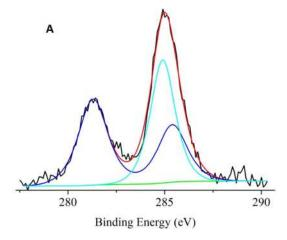
**Figure S5A.** Al  $K\alpha$  excited XPS of the Ru/CeO<sub>2</sub> in the Ru 3d – C 1s energy region; the black line refers to the experimental profile; the green line refers to the background; the peaks at 281.3 and 285.4 eV (blue line) represent the Ru 3d<sub>5/2,3/2</sub> spin-orbit components, the peak at 285.0 eV (cyan line) refers to the adventitious carbon; the red line, superimposed to the experimental profile, refers to the sum of the Gaussian components.
