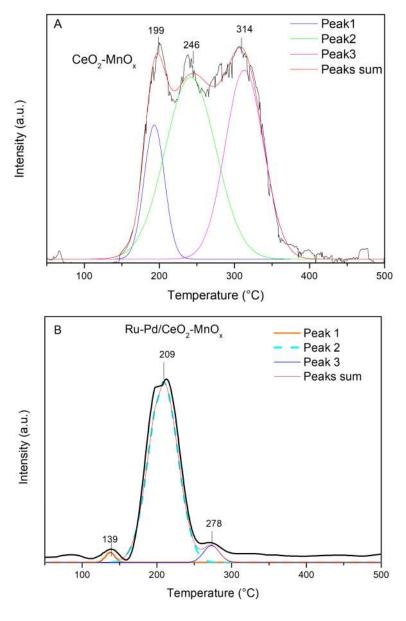
**Figure S1.** H<sub>2</sub>-TPR profiles with peaks deconvolution for Ru/CeO<sub>2</sub>-MnO $_{\times}$  (A) and Ru-Pd/CeO<sub>2</sub>-MnO $_{\times}$  (B) samples.
