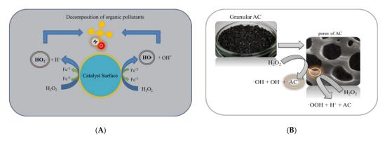
Figure 4. Schematic representation of CWPO mechanism A—catalysed by iron-based materials; B—catalysed by carbon materials (in the absence of iron).
