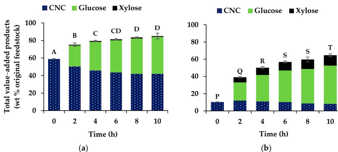
**Figure 2.** Total value-added products (CNC and sugars, wt % original feedstock) extracted from (a) filter paper and (b) wood pulp, via enzyme-mediated CNC production process. Error bars represent standard deviation of the total value-added products (wt % original feedstock). Bars that are denoted by non-identical letters are significantly different ( $p < 0.05$ ). Means and standard
