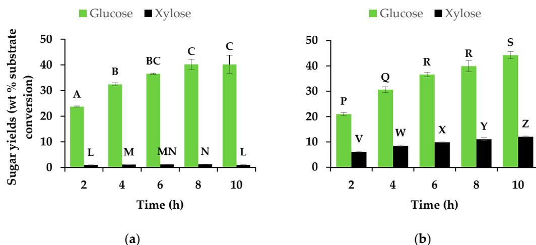
**Figure 1.** Glucose and xylose yields from cellulase cocktail treatment of (a) filter paper and (b) wood pulp over a time period of 2–10 h. Bars that are denoted by non-identical letters within each yield data are significantly different ( $p < 0.05$ ). The cellulase loading for filter paper treatment was calibrated to 1.7 fold higher relative to wood pulp to ensure that enzyme concentration is not a limiting factor based on dosage response curve analysis.
