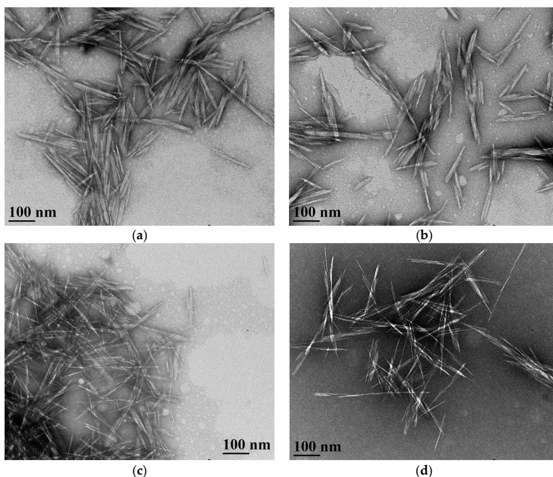
**Figure 3.** Transmission Electron Microscope (TEM) image of CNC isolated from: (a) untreated filter paper; (b) 8 h enzyme-treated filter paper; (c) untreated wood pulp and (d) 8 h enzyme-treated wood pulp.
