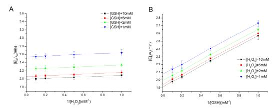
**Figure 1.** Double-reciprocal plots for the reduction of  $H_2O_2$  catalyzed by 6-TediCD in the GSH system. (A)  $[E]_0/v_0$  vs.  $1/[H_2O_2]$  (mM<sup>-1</sup>). (B)  $[E]_0/v_0$  (min) vs. 1/[GSH] (mM<sup>-1</sup>).
