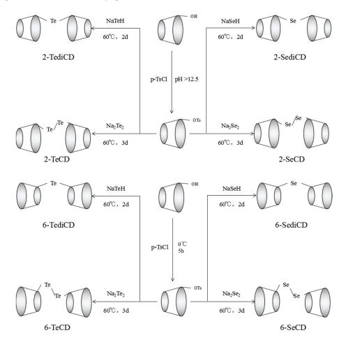
Scheme 1. The synthesis route of 8 types of GPx mimics.
