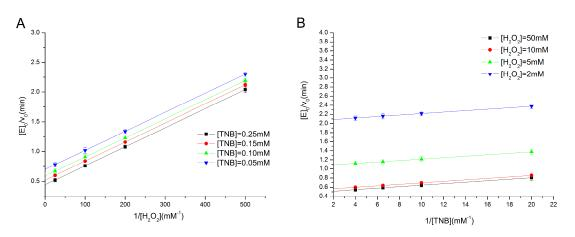
**Figure 2.** Double-reciprocal plots for the reduction of  $H_2O_2$  catalyzed by 6-TediCD in the TNB system. (A)  $[E]_0/v_0$  vs.  $1/[H_2O_2]$  (mM<sup>-1</sup>). (B)  $[E]_0/v_0$  (min) vs. 1/[TNB] (mM<sup>-1</sup>).
