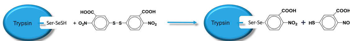
Scheme 6. The absorption equation used to measure the selenium content of the GPx mimic.
