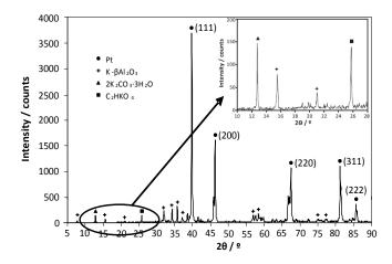
**Figure 4.** XRD spectra after EPOC experiments (CH<sub>3</sub>OH/O<sub>2</sub> = 7.2%/4.6%, 593 K, overnight at -2 V) of a Pt film prepared by impregnation on a K- $\beta$ Al<sub>2</sub>O<sub>3</sub> solid electrolyte. Reprinted with permission from Ref. [31].
