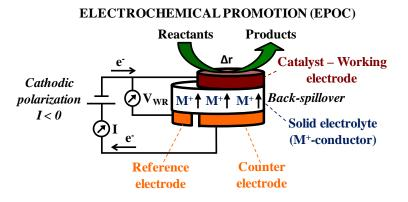
**Figure 1.** Scheme of the electrochemical cell used in electrochemical promotion studies with an alkaline ionic conductor (generally indicated as *M*<sup>+</sup>-conductor) solid electrolytes.
