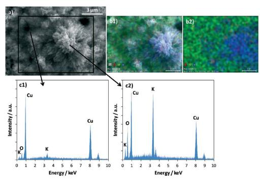
**Figure 3.** Top view SEM image of a selected area of a Cu/K- $\beta$ Al<sub>2</sub>O<sub>3</sub> electrochemical catalyst (**a**) after the EPOC experiments (593 °C, CH<sub>3</sub>OH/O<sub>2</sub> = 4.4%/0.3%,  $V_{WR}$  = -0.5 V for 1 h), along with the corresponding elemental mapping (**b1** and **b2**) of Cu (green), K (blue), and N (red) and the EDX spectra from different regions (**c1** and **c2**). Reprinted with permission from Ref. [32].
