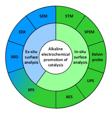
**Figure 2.** Scheme of the different surface analysis techniques used for investigating alkaline Electrochemical Promotion effect.
