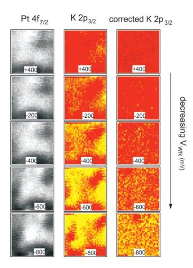
**Figure 7.** Pt 4f7/2 and K 2p3/2 photoelectron intensity maps taken on a Pt/K- $\beta$ Al<sub>2</sub>O<sub>3</sub> catalyst as a function of  $V_{WR}$  at 473 K during the selective hydrogenation of acetylene. Reprinted with permission from Ref. [38].
