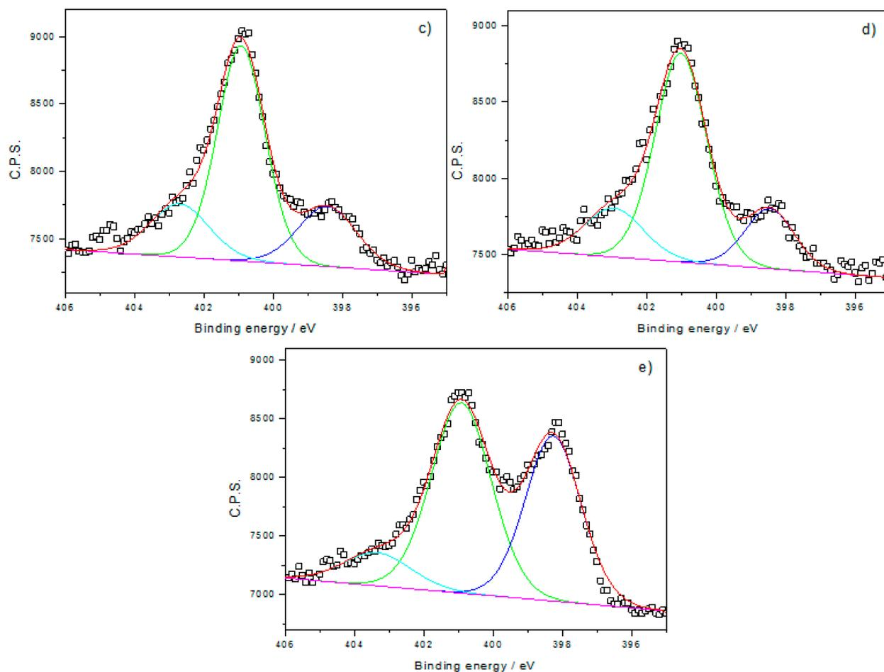
**Figure 2.** N 1s peak and the peak fitting results of the following materials: (a) C-PA-800; (b) C-PA-900; (c) C-PA-1000; (d) C-PA-1100; and (e) C-PA-1000-NH<sub>3</sub>. The unit of y-axis unit is counts per second (C.P.S.).
