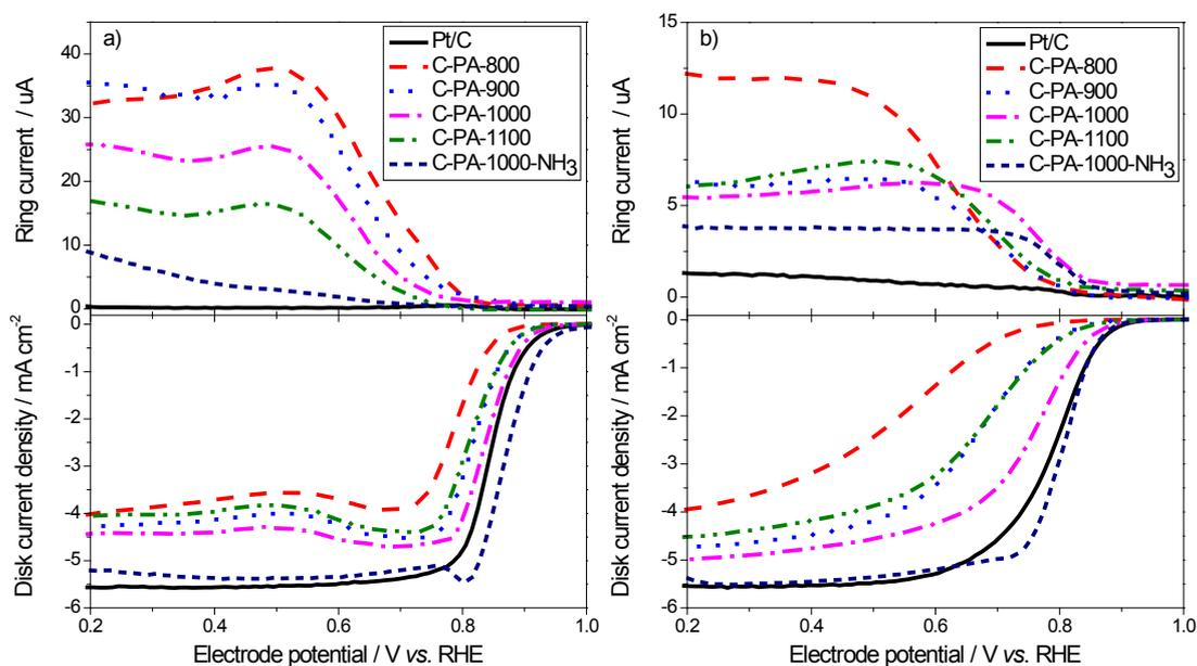
**Figure 4.** Ring (top) and disk (bottom) currents for the RRDE tests of the carbon materials: (a) O<sub>2</sub>-saturated 0.10 M KOH solution; (b) O<sub>2</sub>-saturated 0.10 M HClO<sub>4</sub> solution.
