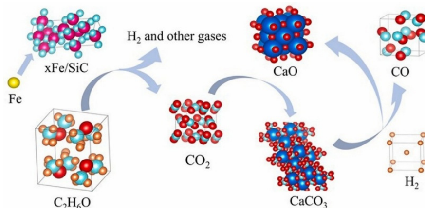
Figure 20. Reforming and hydrogenation–reduction reaction flow [88].
