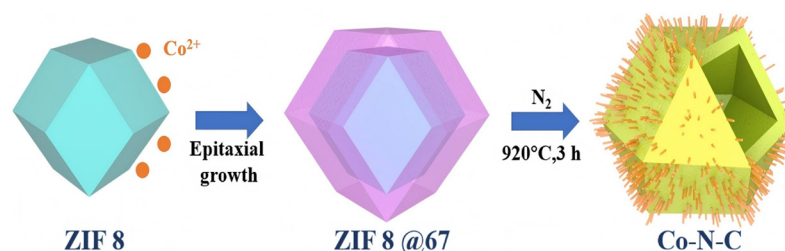
Figure 8. Schematic illustration of the formation process of Co-N-C nanocages [83].
