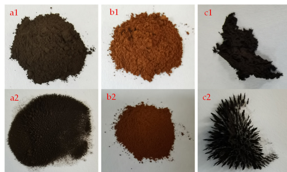
Figure 1. Catalyst morphology and changes caused by magnetic adsorption of ns- \text{Fe}_3\text{O}_4 (a1,a2), \text{Fe}_2\text{O}_3 catalytic material (b1,b2), and \alpha\text{-FeOOH} catalytic material (c1,c2).
