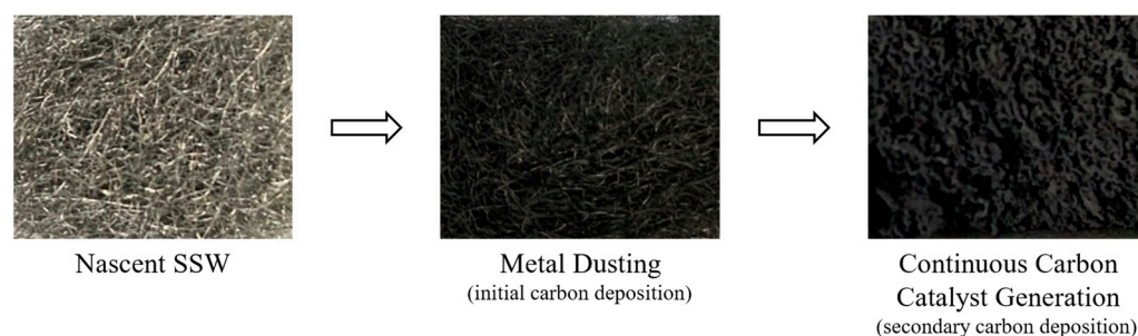
Figure 1. Representation of the 2-stage catalytic TCD process.
