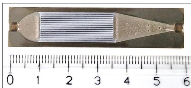
**Figure 1.** Photograph of a catalyst-coated reactor before assembly. The scale is in cm.
