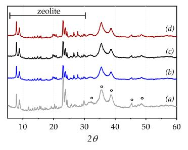
**Figure 2.** XRD patterns upon calcination of: (**a**) parent HYB catalyst; (**b**) HYB-PEI; (**c**) HYB-HPMC; (**d**) HYB-MC. The circles indicate the peaks selected for the determination of crystallinity.
