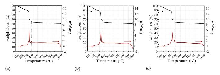
**Figure 1.** TG/DSC curves of the dried binder-containing powders: (**a**) HYB-PEI; (**b**) HYB-HPMC; (**c**) HYB-MC.
