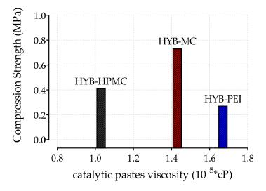
Figure 6. Compression strength of the final monoliths as a function of the paste viscosity.
