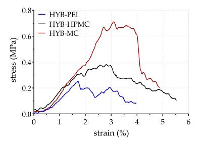
Figure 5. Compressive stress-strain curves for HYB-PEI, HYB-HPMC and HYB-MC monoliths.
