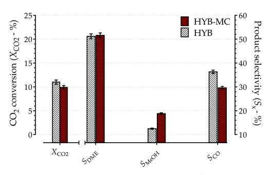
**Figure 7.** Activity–selectivity data during the one-pot hydrogenation of CO<sub>2</sub> to DME ( $P_R$ , 3.0 MPa;  $T_R$ , 220 °C; CO<sub>2</sub>/H<sub>2</sub>/N<sub>2</sub>, 3/9/1 v/v; GHSV: 1000 NL/Kg<sub>cat</sub>/h).
