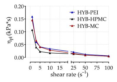
Figure 4. Apparent viscosity of the catalytic pastes as a function of shear rate at 18 °C.
