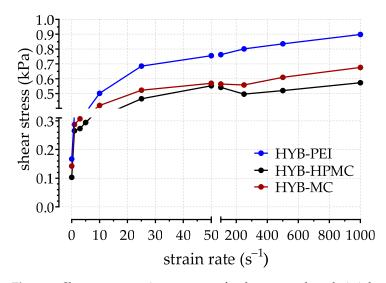
**Figure 3.** Shear stress–strain rate curves for the prepared catalytic ink pastes: HYB-PEI, HYB-HPMC and HYB-MC.
