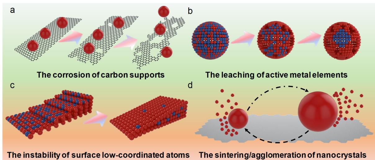
**Figure 2. Illustration schemes of dominant limitations of traditional Pt-based catalysts for ORR.**
