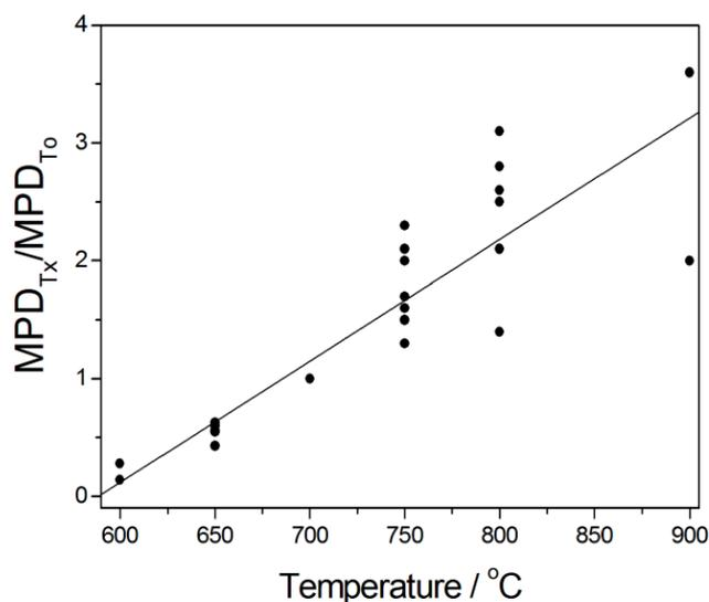
**Figure 12.** The dependence of the ratio of  $x$  °C ( $T_x$ ) to 700 °C ( $T_0$ ) temperature maximum power density ( $MPD_{T_x}/MPD_{T_0}$ ) of hybrid direct carbon fuel cells on cell temperature from data in Table 2.
