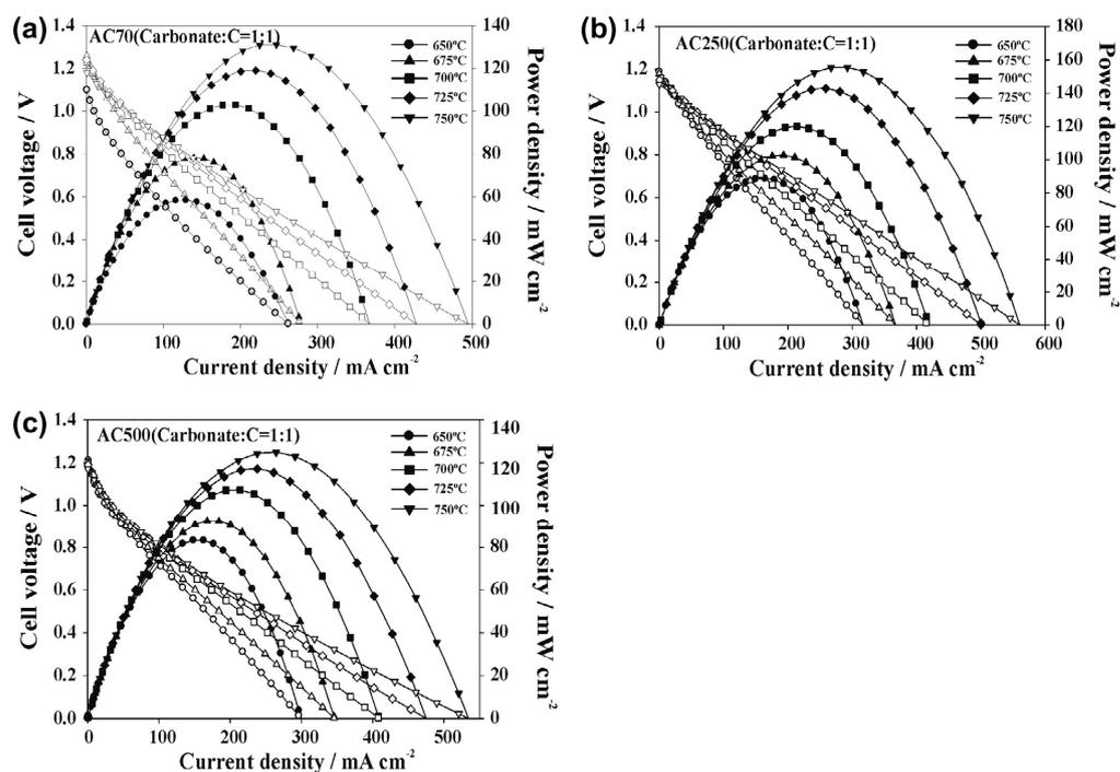
**Figure 9.** Different carbon fuel cell performances with different sizes of activated carbon fuels. Reproduced from Ref. [84], copyright 2013, with permission from Elsevier. (a) AC70; (b) AC250; (c) AC500.
