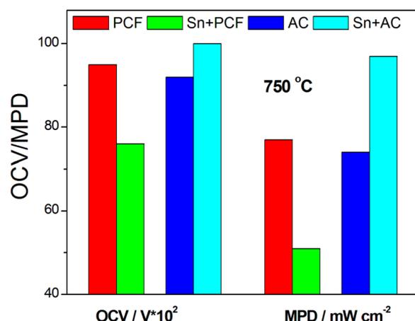
**Figure 4.** The histogram of open-circuit voltage (OCV) and maximum power density (MPD) of the solid oxide–direct carbon fuel cell (SO-DCFC) fueled with lignite (PCF) and activated carbon (AC) without and with Sn presence from data in Ref. [33]. \* is a multiplication sign.
