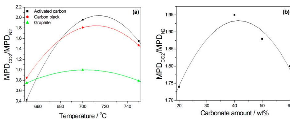
**Figure 11.** (a) Dependence of the ratio of the maximum power density (MPD) with  $CO_2$  purge gas to the MPD with  $N_2$  purge gas ( $MPD_{CO_2}/MPD_{N_2}$ ) on temperature and various types of fuels from data in Ref. [96]; (b) dependence of the  $MPD_{CO_2}/MPD_{N_2}$  ratio on carbonate amount in the fuel from data in Ref. [101].
