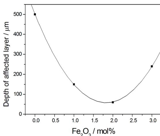
**Figure 5.** Dependence of the depth of affected layer by liquid Sb at 750 °C for 100 h on Fe<sub>2</sub>O<sub>3</sub> content from data in Ref. [43].
