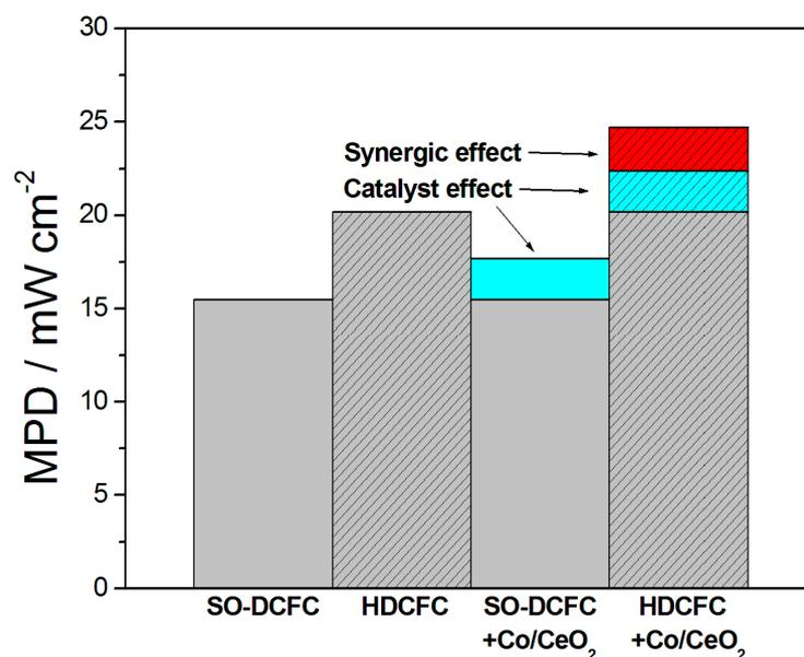
**Figure 10.** Histogram of the maximum power density (MPD) at 800 °C of solid oxide–direct carbon fuel cells (SO-DCFCs) and hybrid direct carbon fuel cells (HDCFCs), with and without catalyst in the fuel from data in Ref. [102].
