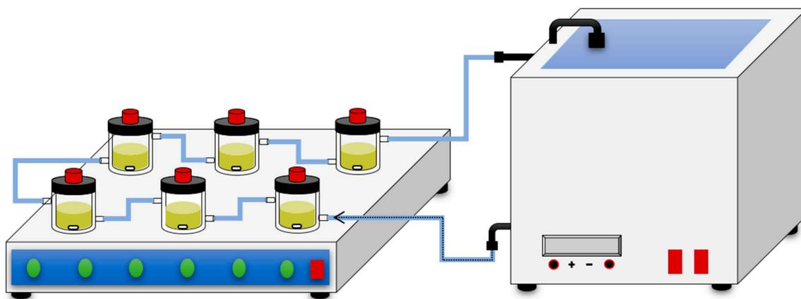
**Figure 6.** Mini reactors used for  $\beta$ -sitosterol oleate production by free and immobilized *C. rugosa* lipase CRL.
