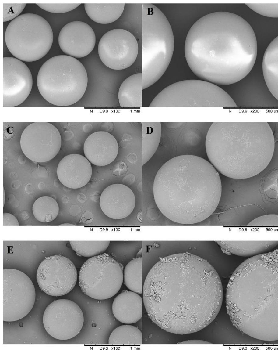
**Figure 1.** Scanning electron microphotographs of (A,B) beads of Lewatit VP OC 1600 ( $\times 100$ ,  $\times 200$ ), (C,D) crude solution of *Y. lipolytica* enzymes immobilized on Lewatit VP OC 1600 ( $\times 100$ ,  $\times 200$ ), and (E,F) liquid lipase Novozym 51032 immobilized on Lewatit VP OC 1600 ( $\times 100$ ,  $\times 200$ ).
