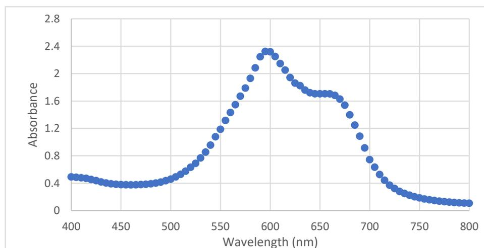
Figure 7. UV–Vis spectrum for derivatives of acetaldehyde.
