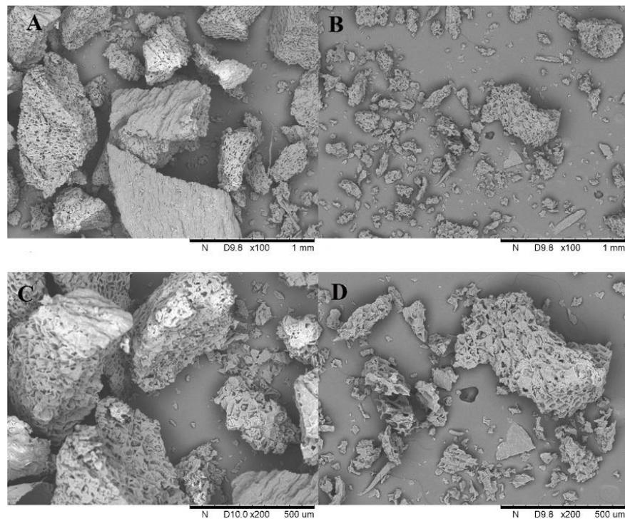
**Figure 3.** Scanning electron microphotographs of (A,C) liquid lipase Novozym 51032 immobilized on coffee grounds ( $\times 100$ ,  $\times 200$ ) and (B,D) coffee grounds ( $\times 100$ ,  $\times 200$ ).
