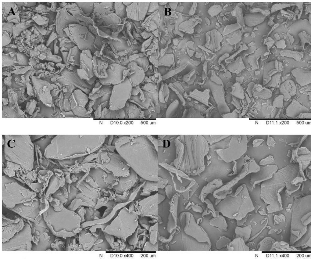
**Figure 2.** Scanning electron microphotographs of (A,C) liquid lipase Novozym 51032 immobilized on chitosan powder ( $\times 200$ ,  $\times 400$ ) and (B,D) chitosan powder ( $\times 200$ ,  $\times 400$ ).
