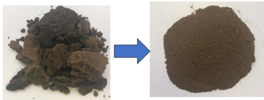
**Figure 5.** Initial and milled to a fraction of 0.1 ÷ 1 mm core material.**Table 4.** Mineral composition of the rock.
