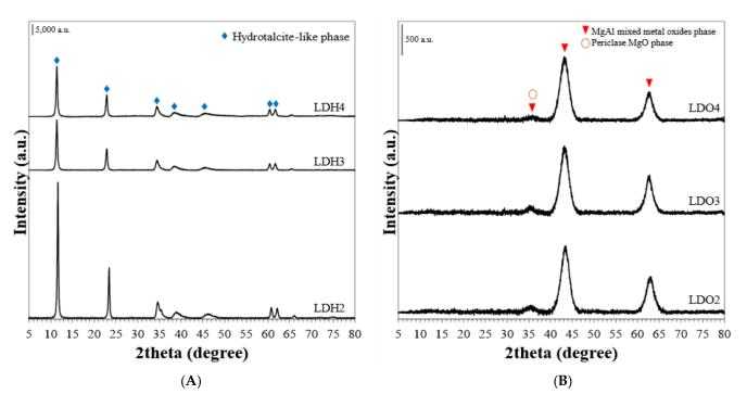
Figure 1. XRD patterns of (A) as-synthesized and (B) calcined LDH samples.
