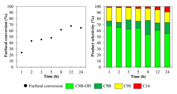
**Figure 5.** Effect of reaction time on furfural conversion and product selectivity obtained from aldol condensation of furfural and 2-butanone over LDO3 catalyst. (Reaction conditions: furfural:2-butanone, 1:5; catalyst loading, 5 wt.%; temperature, 120  $^{\circ}$ C; N<sub>2</sub> pressure, 10 bar).
