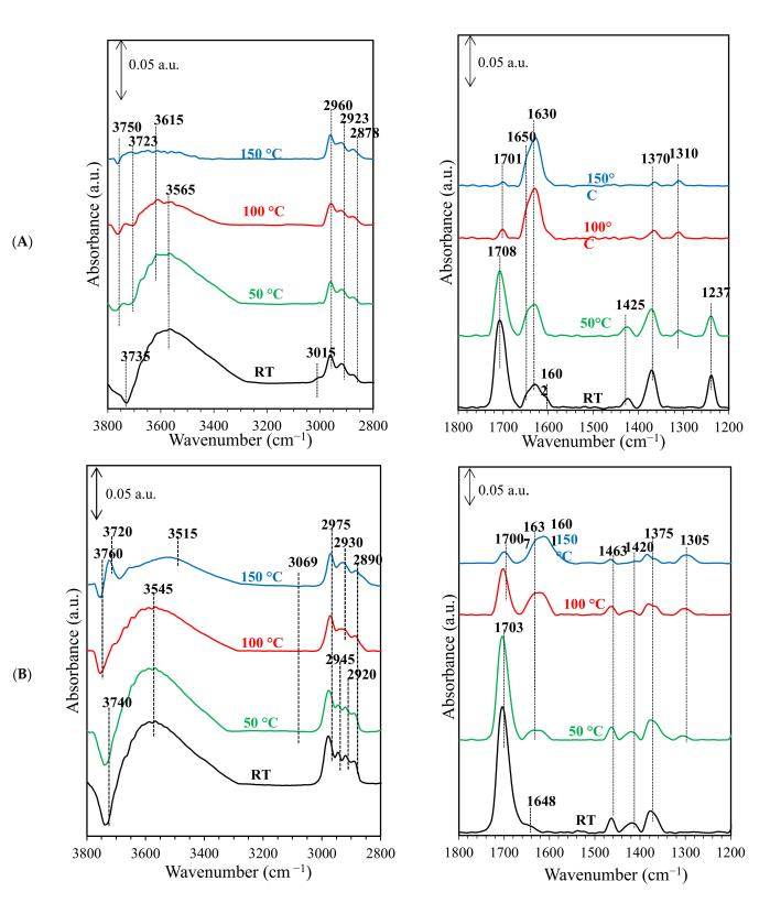
**Figure 9.** In situ FITR spectra of a representative MgAl mixed oxide after the adsorption of (**A**) acetone and (**B**) 2-butanone at room temperature, followed by activation at different temperatures.
