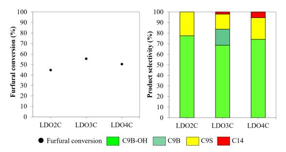
**Figure 4.** Furfural conversion and product selectivity obtained from aldol condensation of furfural and 2-butanone over LDO catalysts with different Mg/Al atomic ratios. (Reaction conditions: furfural:2-butanone, 1:2; catalyst loading, 5 wt.%; time, 8 h; temperature, 80 °C; N<sub>2</sub> pressure, 10 bar).
