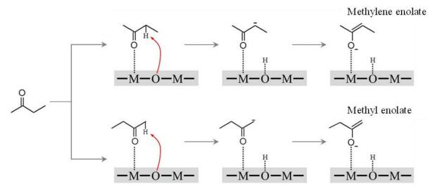
**Figure 3.** Formation of methyl and methylene enolate ions of 2-butonone on medium basic site of metal oxide catalyst.
