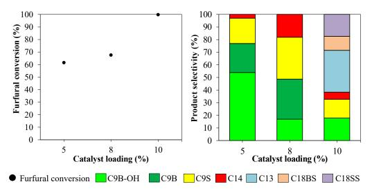
**Figure 7.** Effect of catalyst loading on furfural conversion and product selectivity obtained from aldol condensation of furfural and 2-butanone over LDO3 catalyst. (Reaction conditions: furfural:2-butanone, 1:5; time, 8 h; temperature, 120 °C;  $N_2$  pressure, 10 bar).
