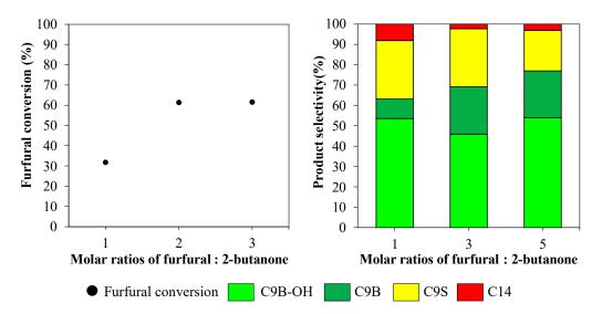
**Figure 6.** Effect of reactants molar ratio on furfural conversion and product selectivity obtained from aldol condensation of furfural and 2-butanone over LDO3 catalyst. (Reaction conditions: catalyst loading, 5 wt.%; time, 8 h; temperature, 80 °C; N<sub>2</sub> pressure, 10 bar).
