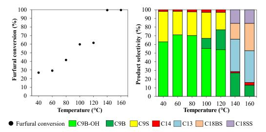
**Figure 8.** Effect of reaction temperature on furfural conversion and product selectivity obtained from aldol condensation of furfural and 2-butanone over LDO3 catalyst. (Reaction conditions: furfural:2-butanone molar ratio, 1:5; catalyst loading, 5 wt.%; time, 8 h; N<sub>2</sub> pressure, 10 bar).
