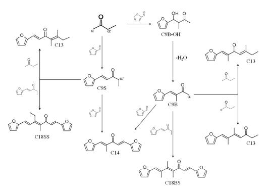
Scheme 1. Proposed reaction pathway for aldol condensation of furfural and 2-butanone over LDO catalyst.
