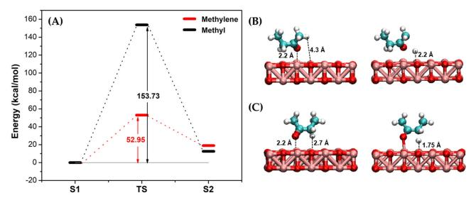
**Figure 10.** (**A**) Energy profile of 2-butanone enolization to generate methylene (red line) and methyl (black line) enolates onto MgO(100) surface, and the stable molecular structures of adsorbed (**B**) methyl and (**C**) methylene enolates, obtained from DFT calculation with M06-2X/6-31G basis set.
