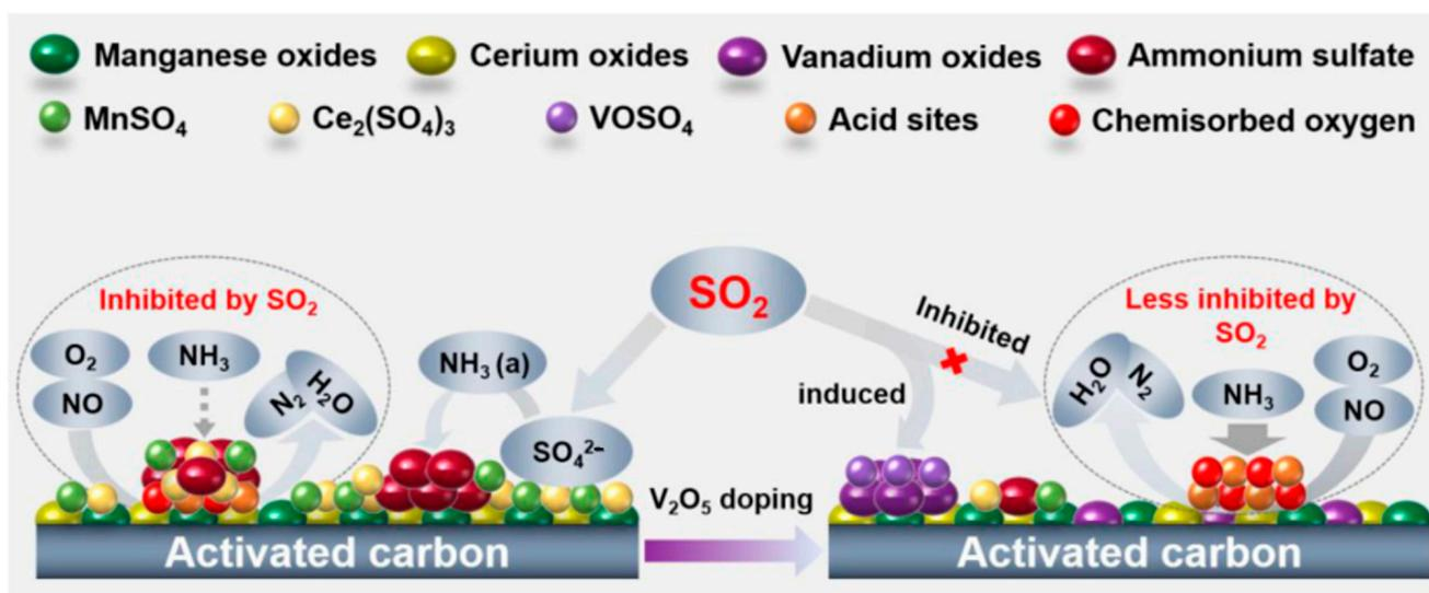
**Figure 8.** Mechanism of  $\text{SO}_2$  tolerance over Mn–Ce(0.4)–V/AC catalysts. (Reproduced with permission from reference [54], Copyright 2019, Elsevier (Amsterdam, The Netherlands)).
