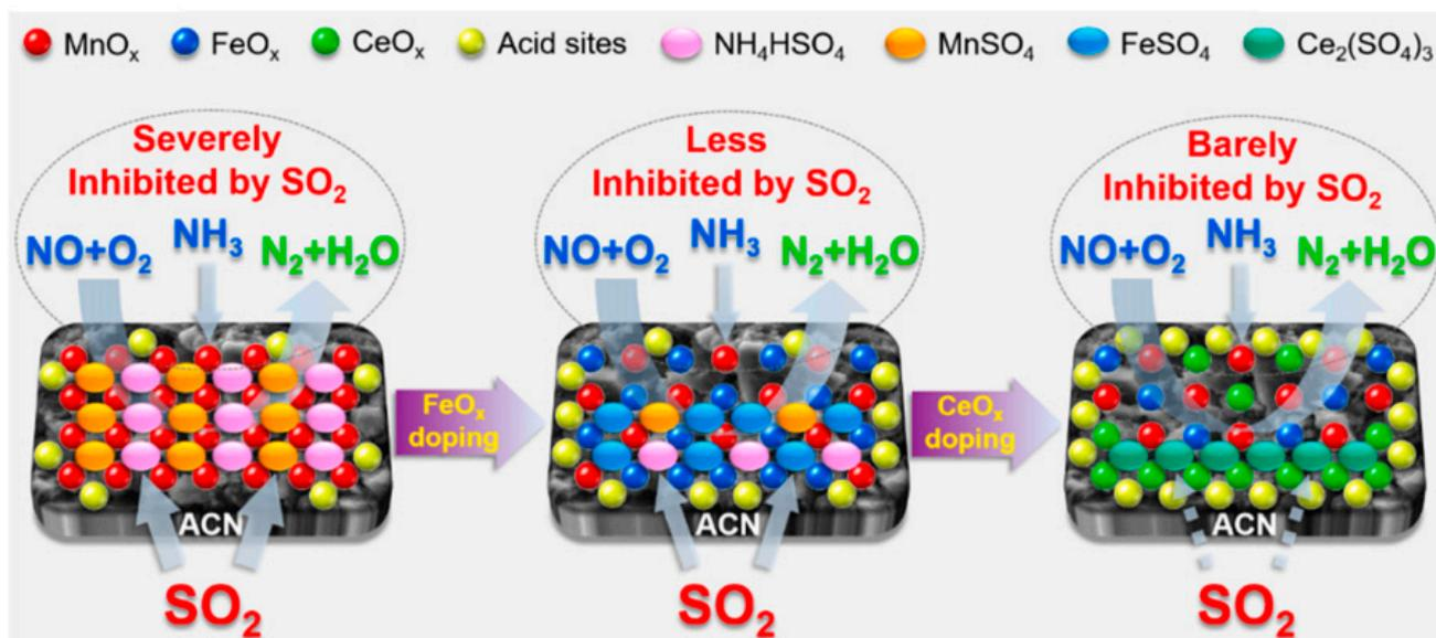
**Figure 18.** Mechanism of better  $SO_2$  tolerance by doping  $FeO_x$  and  $CeO_x$  to Mn/CAN. (Reproduced with permission from reference [95], Copyright 2021, Elsevier (Amsterdam, The Netherlands)).
