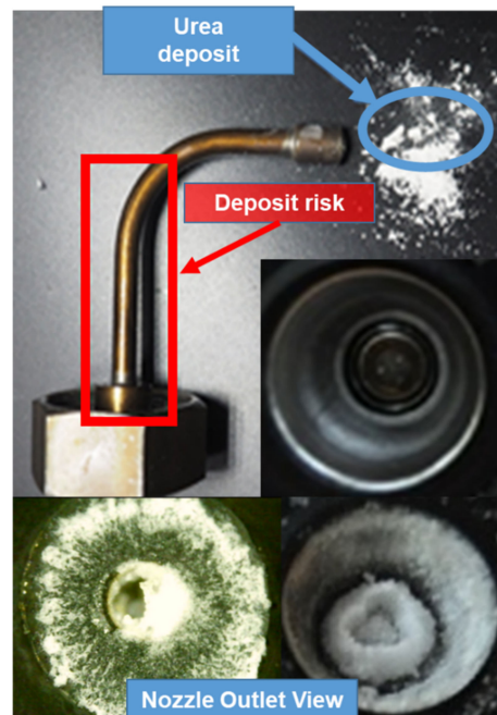
Figure 32. The solid deposit inside the urea injector adapted from Khristamto et al. [39].
