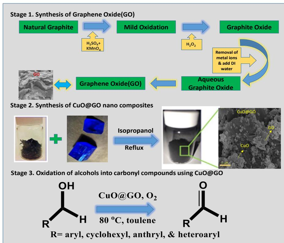
Figure 1. Synthesis of GO, CuO@GO, and oxidation of alcohols into carbonyls (Stages 1, 2 & 3).
