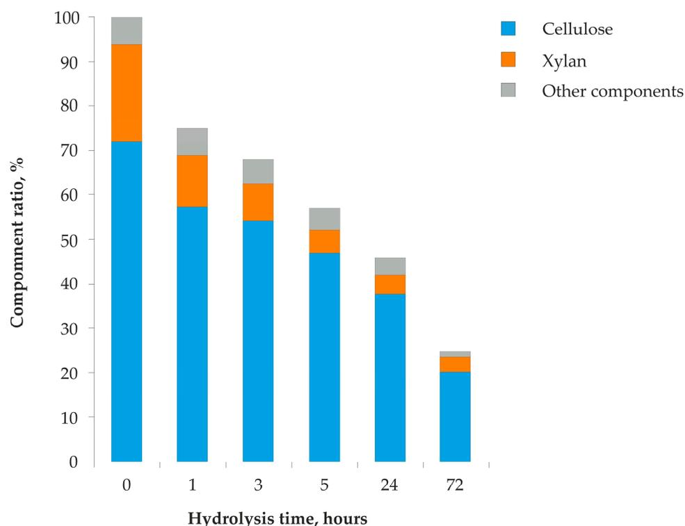
**Figure 1.** Changes in the yield and component composition of biomodified kraft pulp during enzymatic hydrolysis by the *P. verruculosum* complex.
