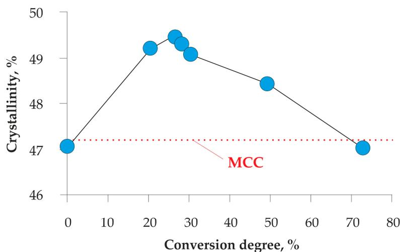
**Figure 4.** Changes in crystallinity of biomodified kraft pulp during enzymatic hydrolysis by *P. verruculosum* cellulases.
