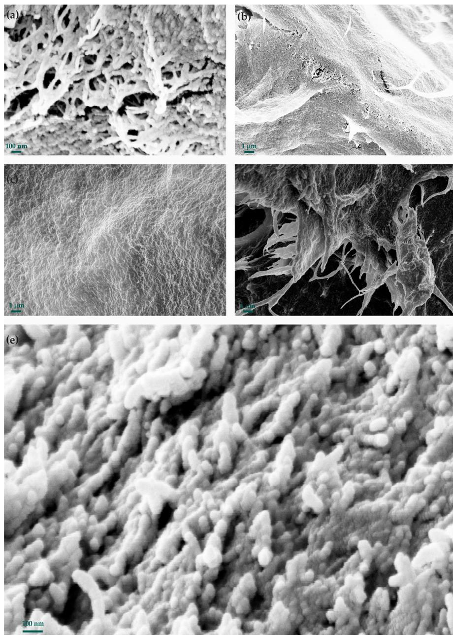
**Figure 3.** SEM images of cryogel samples from initial and biomodified kraft pulps. (a,b)—cryogel samples from initial kraft pulp; (c–e)—cryogel samples from biomodified kraft pulp.
