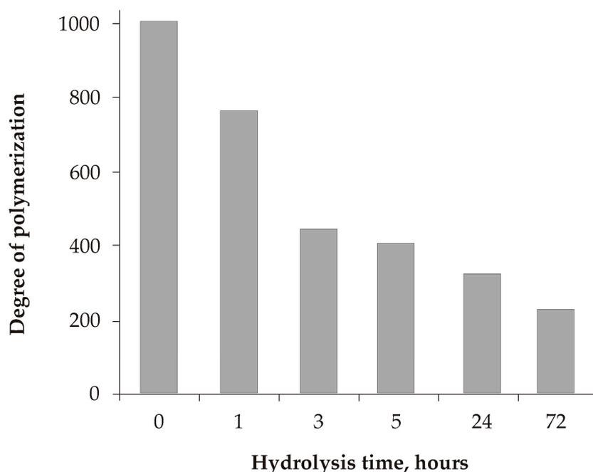
**Figure 2.** Changes in the degree of polymerization of biomodified kraft pulp during biocatalysis.
