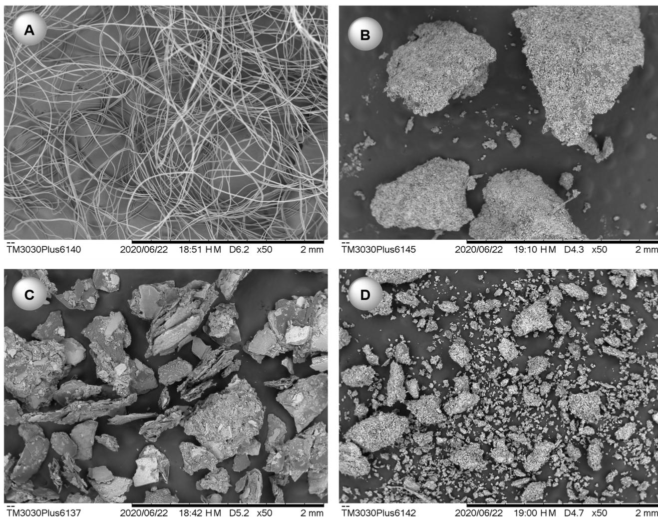
**Figure 3.** Scanning electron microscopy images of silk-fibroin (A), silk-fibroin-Oxone<sup>®</sup> (B), chitin (C), and chitin-Oxone<sup>®</sup> (D).
