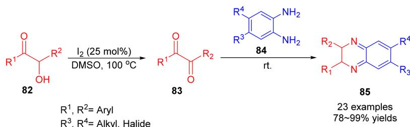
**Scheme 22.** Synthesis of quinoxaline derivatives using iodine as catalyst.
