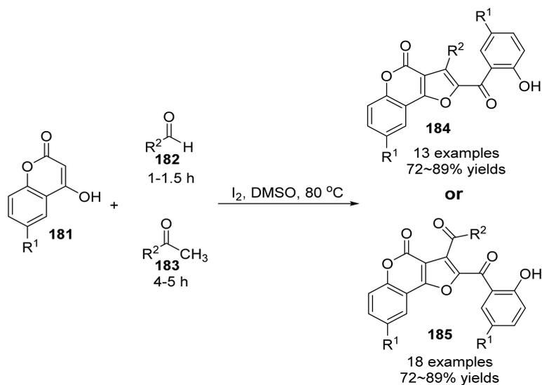
**Scheme 51.** Synthesis of coumarin by  $I_2$ /DMSO-catalyzed synthesis of furan[3,2-c]coumarin.
