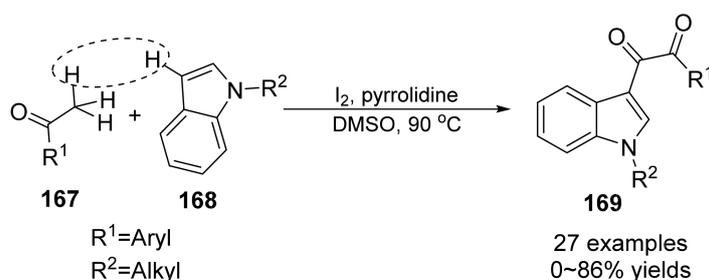
**Scheme 48.** Direct and selective oxidative cross-coupling of indoles with methyl ketones.
