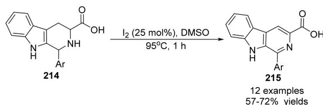
**Scheme 59.** Synthesis of  $\beta$ -carboline-3-carboxylic acids catalyzed by  $I_2$ /DMSO.
