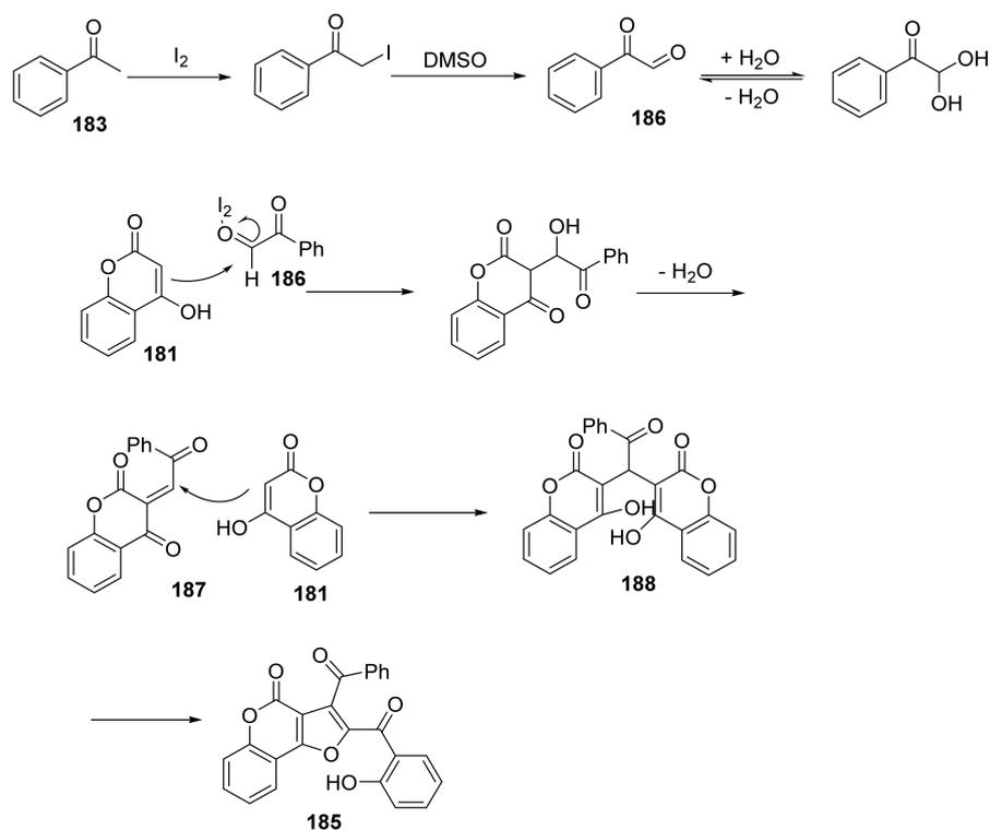
**Scheme 52.** Mechanism for the formation of furo[3,2-c]coumarin **5a**.
