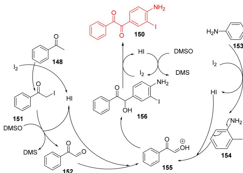
**Scheme 44.** Mechanism of  $I_2$ -catalyzed highly chemical- and site-selective oxidative cross-coupling using acetophenone and aniline.
