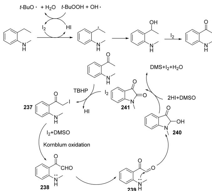
**Scheme 67.** Mechanism of synthesis of isatins catalyzed by  $I_2$ /DMSO.
