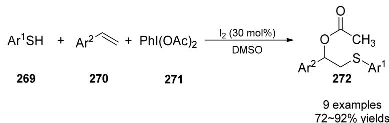
**Scheme 74.** Synthesis of  $\beta$ -acetoxy sulfides by bifunctionalization of olefins catalyzed by  $I_2$ /DMSO.
