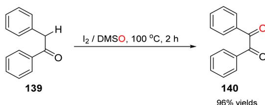
**Scheme 39.**  $I_2$ /DMSO oxidation of benzyl phenyl ketone to benzil.
