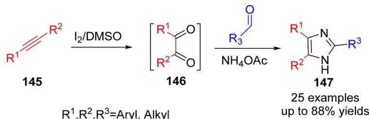
**Scheme 42.** Synthesis of trisubstituted imidazole derivatives by oxidation of alkynes using an  $\text{I}_2/\text{DMSO}$  system.
