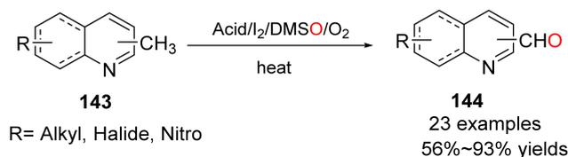
**Scheme 41.** Aerobic oxidation of methyl group on aromatic compound.
