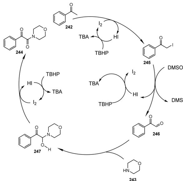
**Scheme 69.** Mechanism of synthesis of 1-morpholine-2-phenyl-1-morpholine-2-Dione from acetophenone and morpholine.
