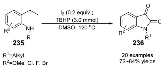
**Scheme 66.** I<sub>2</sub>/TBHP/DMSO Mediated synthesis of isatins from 2-ethylanilines.
