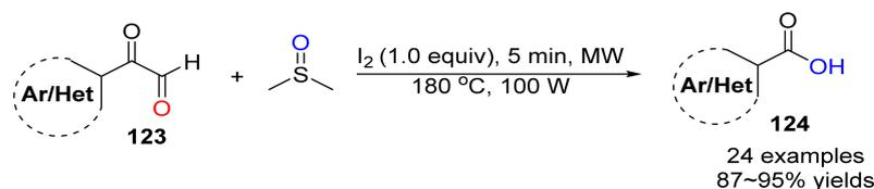
**Scheme 33.** The cleavage of  $\alpha$ -ketoaldehyde catalyzed by  $\text{I}_2/\text{DMSO}$ .
