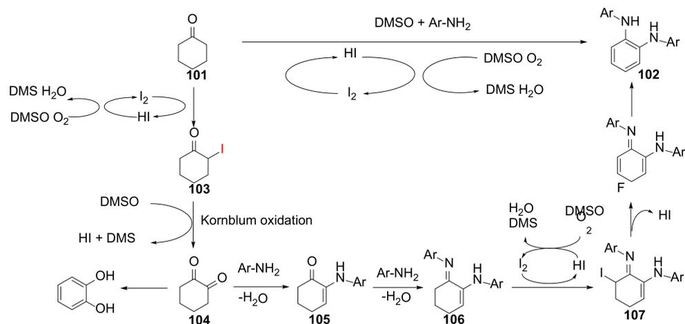
**Scheme 28.** A mechanism of iodine-catalyzed formation of *N,N'*-diaryl-*o*-phenylenediamines.
