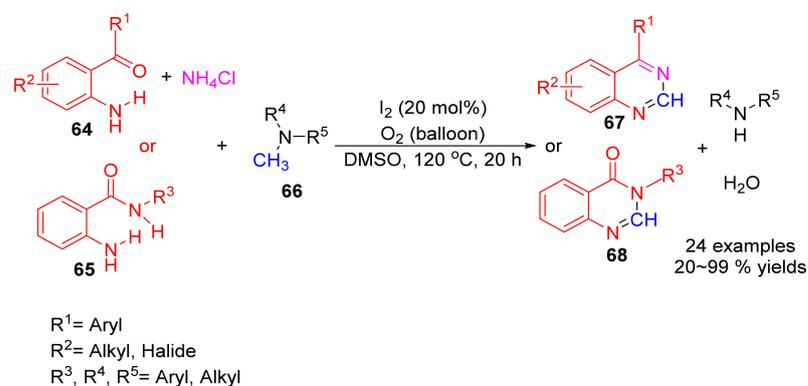
**Scheme 18.** C(sp<sup>3</sup>)-H Bond Activation by iodine Catalytic Oxidation.
