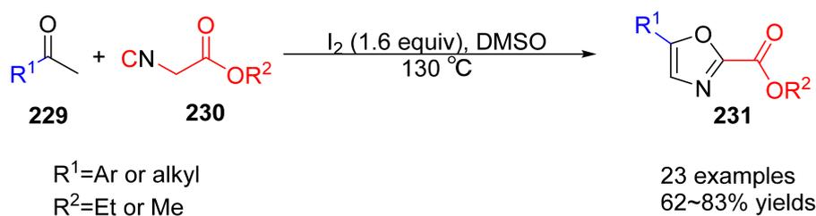
**Scheme 64.** Synthesis of oxazoles by iodine-catalyzed [3 + 2] cycloaddition reaction.
