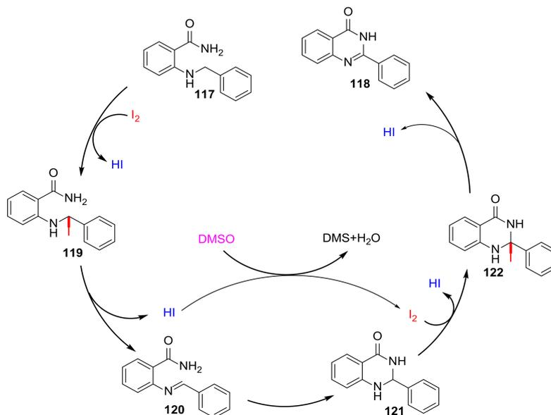
**Scheme 32.** Mechanism of I<sub>2</sub>/DMSO-mediated intramolecular C(sp<sup>3</sup>)-H/N-H oxidative cross-coupling reaction.
