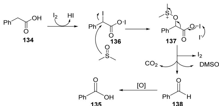
**Scheme 38.** Mechanism of decomposition of phenylacetic acid to benzoic acid.
