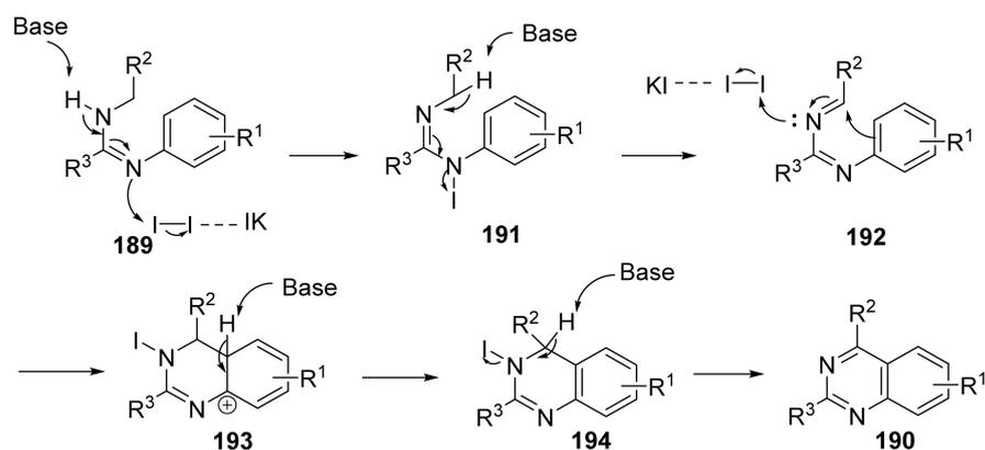
Scheme 54. Reaction mechanism of cyclization to quinazoline.
