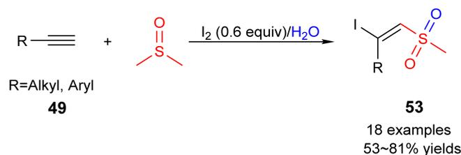
**Scheme 15.** Synthesis of (*E*)- $\alpha$ -Iodo- $\beta$ -methylsulfonylalkenes compounds catalyzed by  $\text{I}_2/\text{DMSO}$ .
