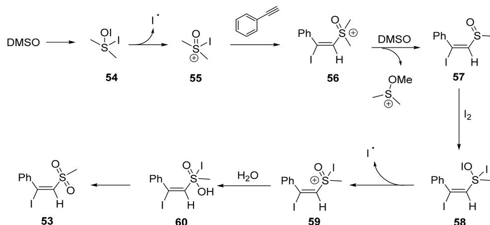
**Scheme 16.** Mechanism of synthesis of (*E*)- $\alpha$ -Iodo- $\beta$ -methylsulfonylalkenes catalyzed by  $I_2$ /DMSO.
