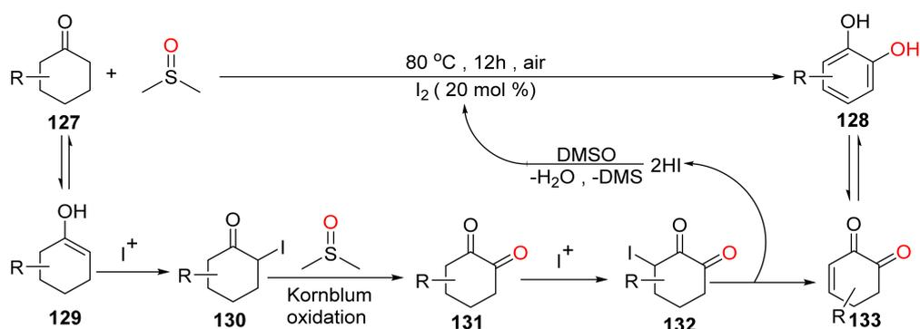
**Scheme 36.** Mechanism of cyclohexanones conversion to catechols.
