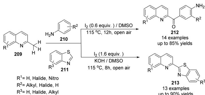
**Scheme 58.** Synthesis of C4-carbonylated aniline (4-aminophenyl)(quinoline-2-yl) methanones and 2-heteroarylbenzothiazoles catalyzed by  $I_2$ /DMSO.
