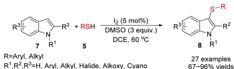
**Scheme 3.** Sulfenylation of indoles by using  $I_2$  as catalyst and DMSO as oxidant.
