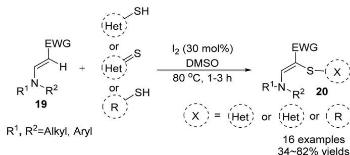
**Scheme 6.** I<sub>2</sub>/DMSO-catalyzed cross dehydrogenative coupling reaction.
