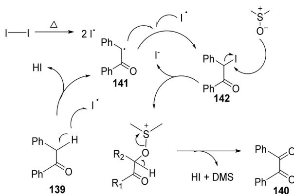
**Scheme 40.** Alpha C–H oxidation of ketone catalyzed by  $I_2$ /DMSO.
