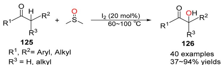
**Scheme 34.**  $\alpha$ -hydroxylation of ketones catalyzed by  $\text{I}_2/\text{DMSO}$ .
