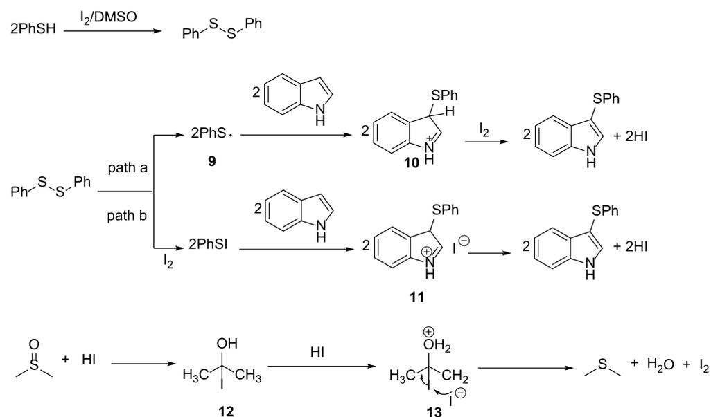
**Scheme 4.** Mechanism of 3-sulfonation of indole.
