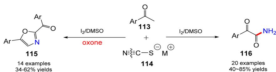
**Scheme 30.** Synthesis of  $\alpha$ -ketoamides and 2-acyloxazoles from arylmethyl ketones and thiocyanates catalyzed by  $I_2$ /DMSO.
