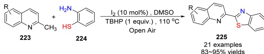
**Scheme 62.** Synthesis of 2-azaarenyl benzothiazoles by catalytic oxidation of I<sub>2</sub>/DMSO.
