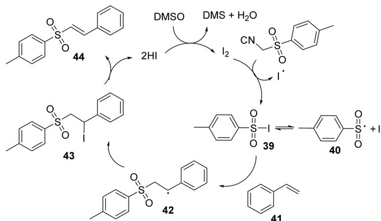
**Scheme 11.** Reaction mechanism of  $I_2$ /DMSO catalytic synthesis of sulfone.
