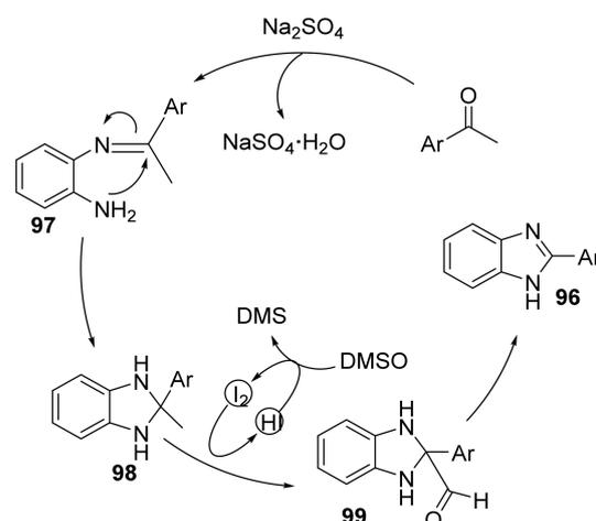
**Scheme 26.** Mechanism of cyclization of aryl alkyl ketones catalyzed by iodine.
