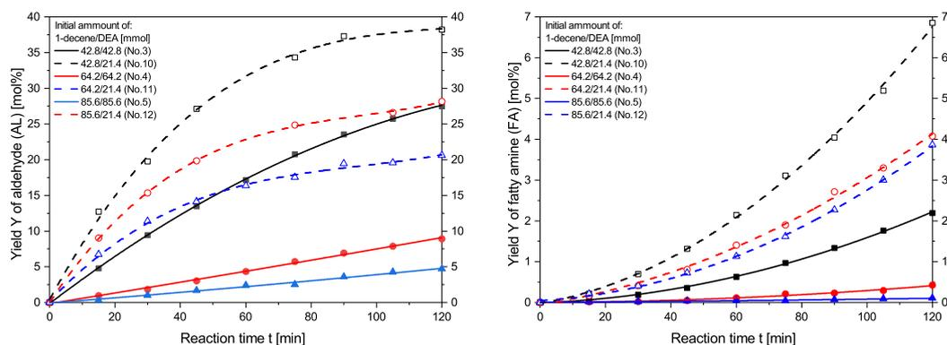
**Figure 5.** Comparison of aldehyde production (left) and fatty amine production (right) depending on initial concentrations of 1-decene and diethylamine. Reaction conditions:  $T = 120\text{ }^{\circ}\text{C}$ ,  $p = 30\text{ bar}$   $\text{H}_2/\text{CO}$  (2:1), 0.23 mol% Rh, 0.92 mol% SX, 12 g organic phase (1-decene + dodecane), 12 g water, 8 wt% Marlophen NP8, 1 wt%  $\text{Na}_2\text{SO}_4$ , 1200 rpm,  $t = 2\text{ h}$ .
