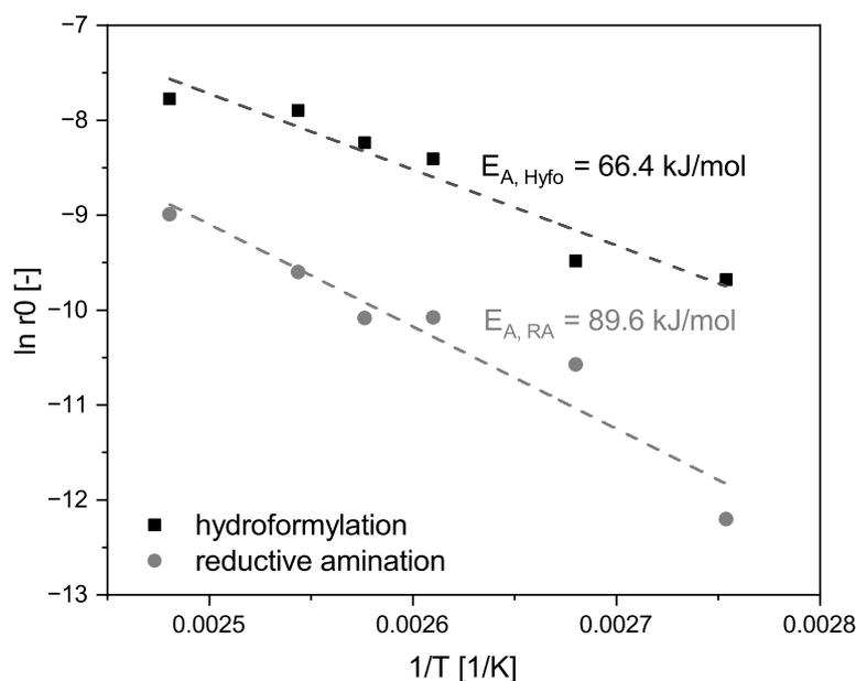
**Figure 3.** Arrhenius diagram for the substep hydroformylation and reductive amination.
