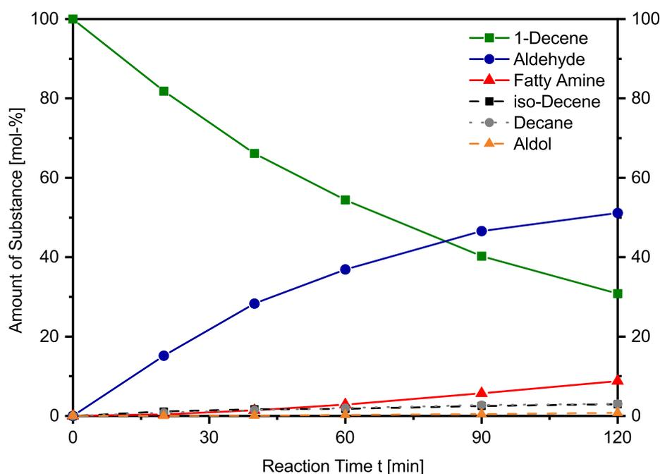
**Figure 2.** Concentration profile for the hydroaminomethylation of 1-decene with diethylamine in an aqueous microemulsion system. Reaction conditions:  $p = 30$  bar  $H_2/CO$  2:1, 0.23 mol% Rh, 0.92 mol% SX, 21.4 mmol 1-decene, 21.4 mmol DEA, 9 g dodecane (co-solvent), 12 g water, 8 wt% Marlophen NP8, 1 wt%  $Na_2SO_4$ , 1200 rpm,  $t = 4$  h.
