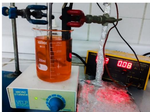
**Figure 8.** Experimental instrument used in the Electro-Fenton process.
