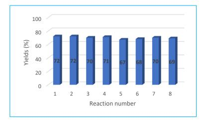
**Figure 3.** Use of  $MoO_2Cl_2(H_2O)_2$  in consecutive reductive depolymerizations of P4HB. The reactions were carried out using  $MoO_2Cl_2(H_2O)_2$  (5 mol%) by successive additions of P4HB (0.5 mmol) and TMDS (1.5 mmol) to the reaction mixture, without separating the catalyst at the end of each reaction. Yields were determined by <sup>1</sup>H NMR spectroscopy, using mesitylene as an internal standard.
