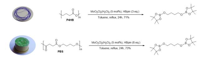
**Scheme 1.** Reductive depolymerization of P4HB and PBS waste with the system  $MoO_2Cl_2(H_2O)_2/HBpin$ .
