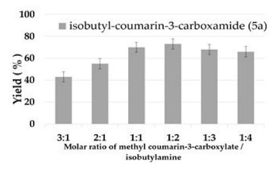
**Figure 3.** The effect of the molar ratio on the enzymatic synthesis of coumarin carboxamide derivative under continuous-flow conditions.
