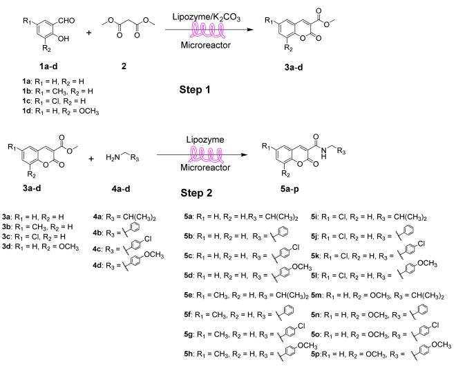
Scheme 1. Synthesis of coumarin carboxamide derivatives in the continuous flow microreactors.
