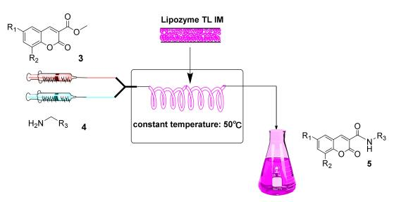
**Figure 6.** Experimental setup for coumarin carboxamide derivative synthesis in microreactors catalyzed by lipase TL IM.
