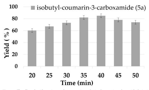
**Figure 4.** The effect of residence time on the enzymatic synthesis of coumarin carboxamide derivative under continuous-flow conditions.
