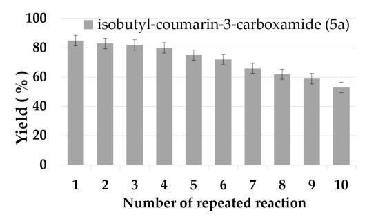
**Figure 5.** The effect of enzyme reusability on the enzymatic synthesis of coumarin carboxamide derivative under continuous-flow conditions.
