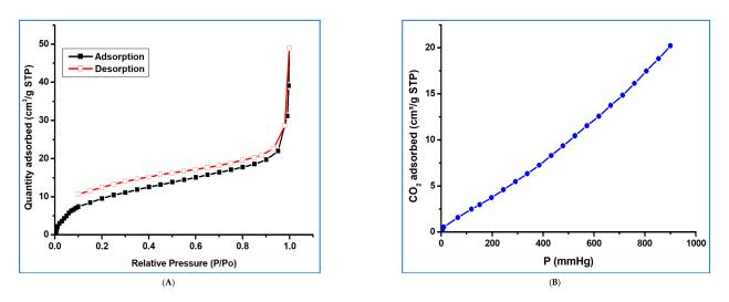
Figure 1. (A) N<sub>2</sub> sorption isotherm of framework 1 at 77 K. (B) CO<sub>2</sub> sorption isotherm of 1 at 273 K.
