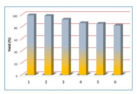
**Figure 4.** Yield of 2-benzylidenemalononitrile (**D**) upon catalyst recycling for the deacetalization– Knoevenagel reactions catalyzed by CP **1**.
