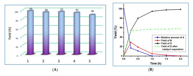
**Figure 3.** (**A**) Yields of 2-benzylidenemalononitrile by using CPs **1–5** as catalysts. (**B**) Yield vs. time plot for the deacetalization–Knoevenagel condensation reactions catalyzed by CP **1** (black line: yield of 2-benzylidenemalononitrile (**D**); red line: yield of benzaldehyde (**B**); blue line: percentage of unreacted benzaldehyde dimethyl acetal (**A**); dotted green line: yield of 2-benzylidenemalononitrile (**D**) upon separating the catalyst after 0.25 h of reaction time).
