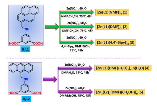
Scheme 2. Synthesis of coordination polymers 1–5 by reactions of  $H_2L1$  and  $H_2L2$  with  $Zn(NO_3)_2 \cdot 6H_2O$  under various solvothermal conditions.
