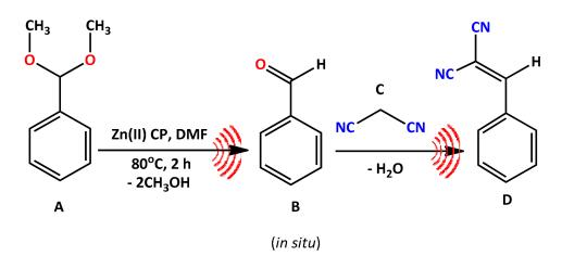
Scheme 1. One-pot cascade deacetalization–Knoevenagel condensation reaction catalyzed by 1–5 Zn(II) coordination polymers (A—benzaldehyde dimethylacetal; B—benzaldehyde; C—malononitrile; D—2-benzylidenemalononitrile).
