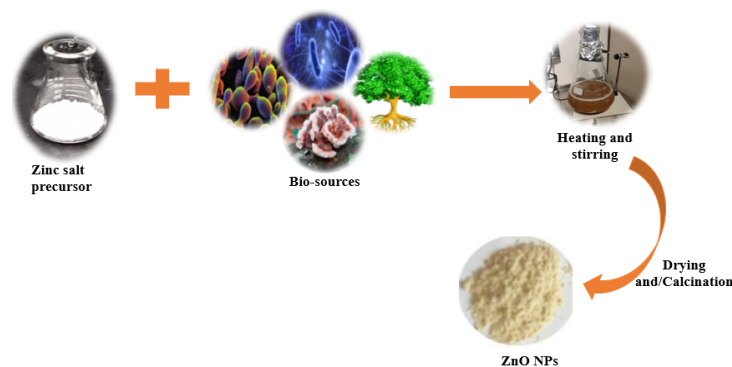
Figure 3. Schematic representation for the green synthesis of ZnO nanoparticles.
