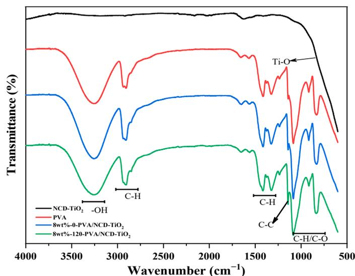
Figure 3. ATR/FTIR spectra of various samples.
