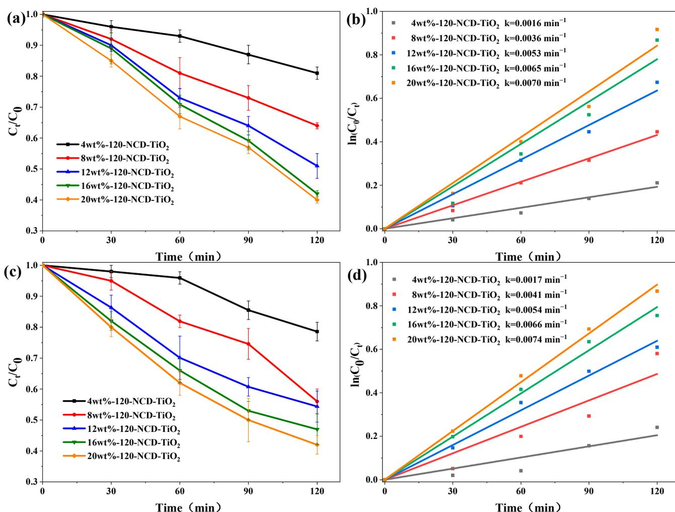
**Figure 6.** Photocatalytic activities of PVA/NCD-TiO<sub>2</sub> nanocomposite films with various concentrations of NCD-TiO<sub>2</sub> on the degradation of phenol (a,b) and LEV (c,d) under visible-light irradiation.
