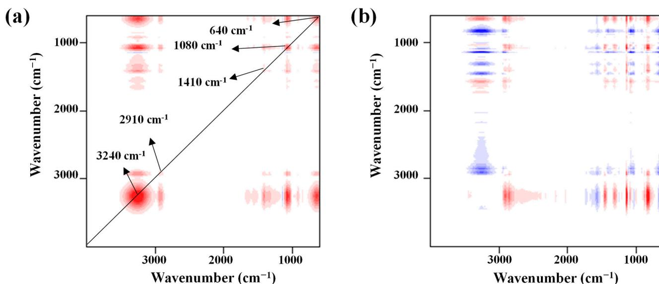
**Figure 4.** 2DCOS analysis diagram of PVA/NCD-TiO<sub>2</sub>. (a) Synchronous spectral analysis and (b) asynchronous spectral analysis.
