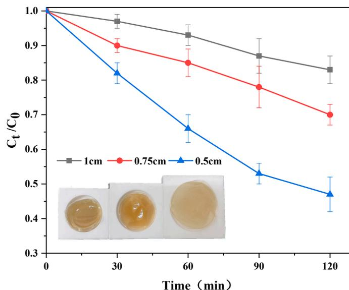
**Figure 7.** Photocatalytic activity of the PVA/NCD-TiO<sub>2</sub> nanocomposite films fabricated with different thicknesses for LEV removal under visible light.
