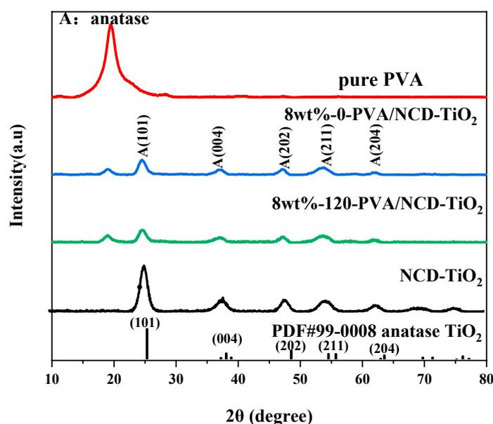
Figure 2. XRD spectra of pure PVA, 8 wt%-0-PVA/NCD-TiO<sub>2</sub>, and 8 wt%-120-PVA/NCD-TiO<sub>2</sub>.
