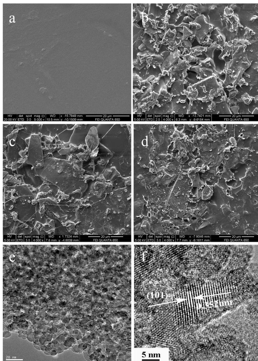
**Figure 1.** SEM images of the surfaces of (a) pure PVA, (b) 8 wt%-0-PVA/NCD-TiO<sub>2</sub>, (c) 8 wt%-120-PVA/NCD-TiO<sub>2</sub>, and (d) 8 wt%-160-PVA/NCD-TiO<sub>2</sub>; TEM images of (e,f) the NCD-TiO<sub>2</sub> nanoparticle.
