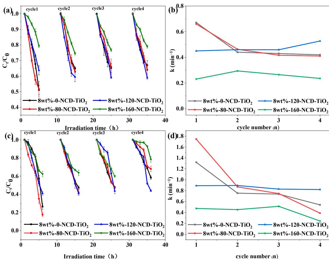
**Figure 5.** (a) Degradation of phenol and (b) the reaction rate constant  $k$  for the photocatalytic degradation of phenol during four cycles in the presence of the PVA/NCD- $\text{TiO}_2$  hybrid films treated at different temperatures; (c) degradation of LEV and (d) the reaction rate constant  $k$  for the photocatalytic degradation of LEV during four cycles in the presence of the PVA/NCD- $\text{TiO}_2$  hybrid films treated at different temperatures.
