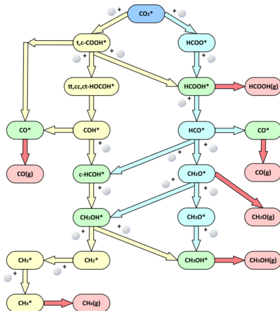
Figure 2. The possible reaction networks of CO 2 hydrogenation to CO, HCOOH, CH 2 O, CH 3 OH, and CH 4 at the TaC (111) surface. It should be noted that the adsorbed intermediates on the surface are indicated by the symbol *.
