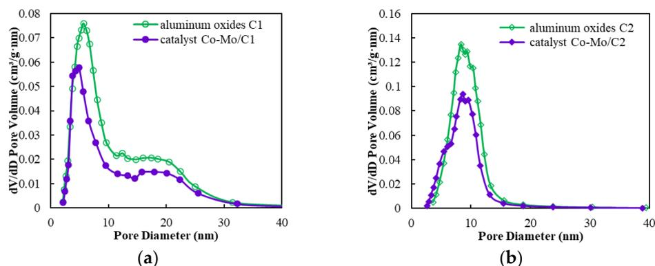
**Figure 5.** (a) Pore size distribution for aluminum oxides C1 and catalysts. (b) Pore size distribution for aluminum oxides C2 and catalysts.
