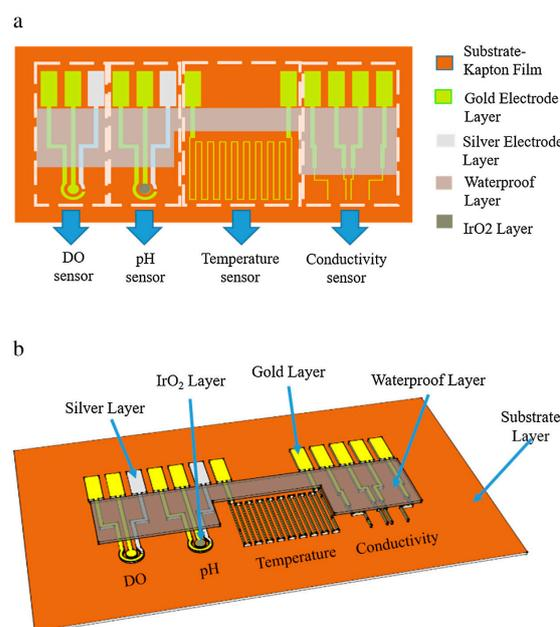
**Figure 1.** Image of dissolved oxygen (DO), pH, temperature, and conductivity MEA sensors (a) and layers on each MEA sensor (b). Reprinted with permission from Ref. [21]. (Copyright, 2016, Elsevier).
