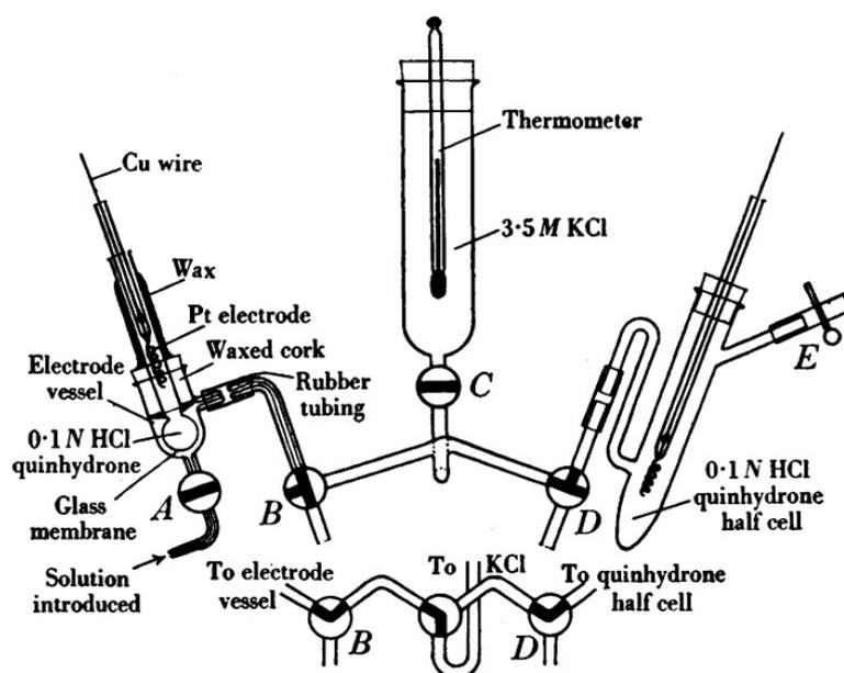
Figure 4. The design of glass electrode measurement, reprinted with permission from reference [57]. (Copyright, Portland Press, 1933).
