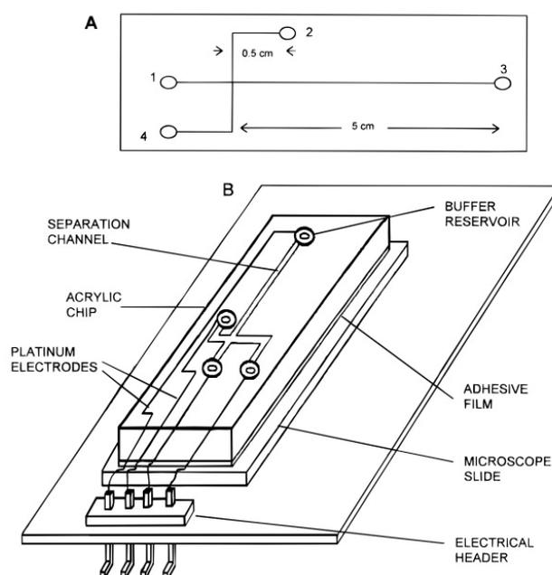
**Figure 10.** Design of the plastic microchannel chip (A) and ichnography (B) the details of the completed chip. Reprinted with permission from reference [152]. (Copyright, 1997, American Chemical Society).
