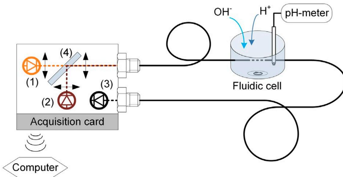
**Figure 6.** The specific structure of optical fiber pH sensor and its experimental design. (1) Signal light source (2) referred light source (3) photodiode and (4) dichroic mirror, reprinted with permission from reference [83]. (Copyright, Elsevier, 2014).
