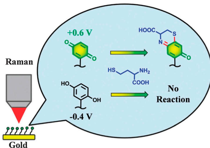
**Figure 5.** The mechanism of quinone hydroquinone-SAM on a gold electrode surface. Reprinted with permission from Ref. [68]. (Copyright, ACS, 2013).
