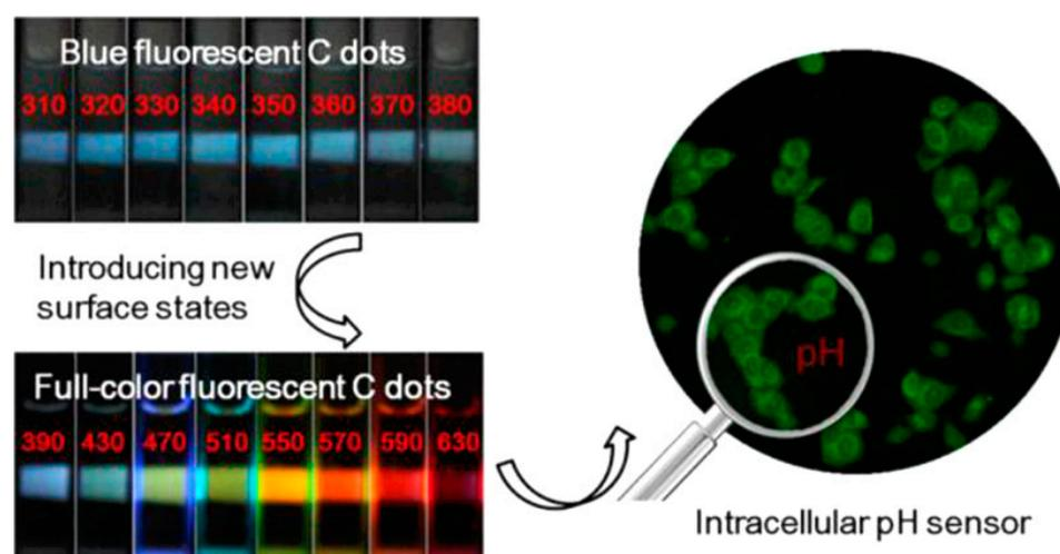
**Figure 2.** The integration of carbon dots with different adjusted full-color emission and pH sensors. Reprinted with permission from Ref. [34]. (Copyright, 2014 ACS).
