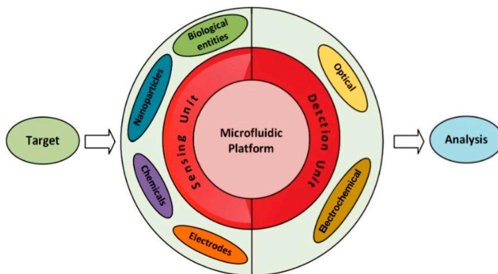
**Figure 8.** The diagram of a microfluidic sensing system. Reprinted with permission from Ref. [127]. (Copyright, 2019, MDPI).
