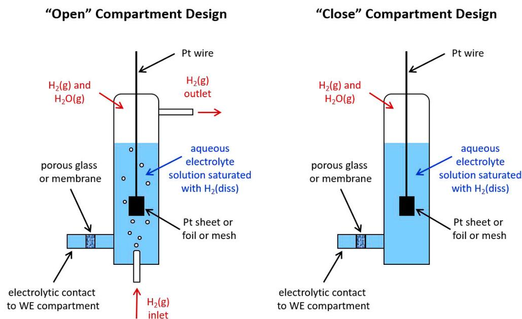
**Figure 3.** "Open" and "close" designs of the reference electrode compartment of the hydrogen reference electrode, reprinted with permission from reference [56]. (Copyright, ACS, 2020).
