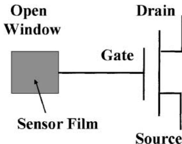
**Figure 7.** Integral diagram of the discrete ISFET. Reprinted with permission from Ref. [90]. (Copyright, 2001, Elsevier).
