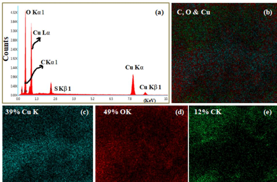
Figure 3. (a) EDAX analysis and (b–e) EDS mapping of the synthesized rGO-CuO composite.
