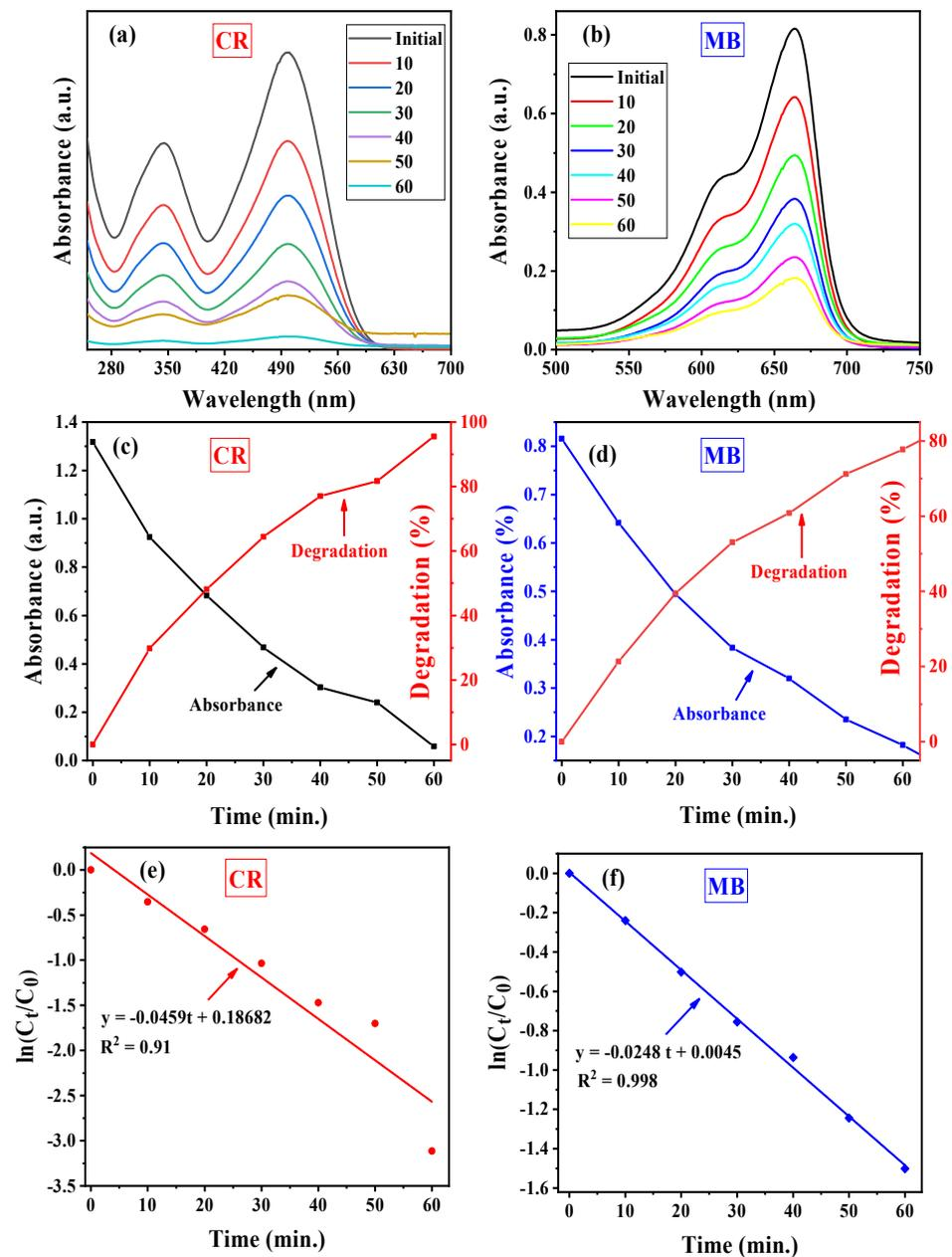
**Figure 6.** Decrease in absorption intensity with time (a,b), absorbance and degradation percentage (c,d) and kinetics plots (e,f) for the degradation of CR and MB dyes, respectively, in 1 h of irradiation under visible light utilizing rGO-CuO nanocomposites as a catalyst.
