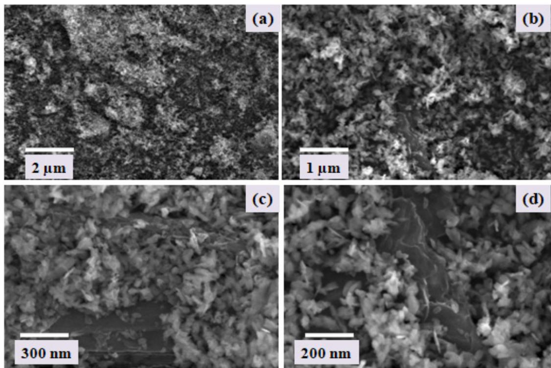
Figure 2. FESEM images of (a–d) rGO-CuO nanocomposites with different magnifications.
