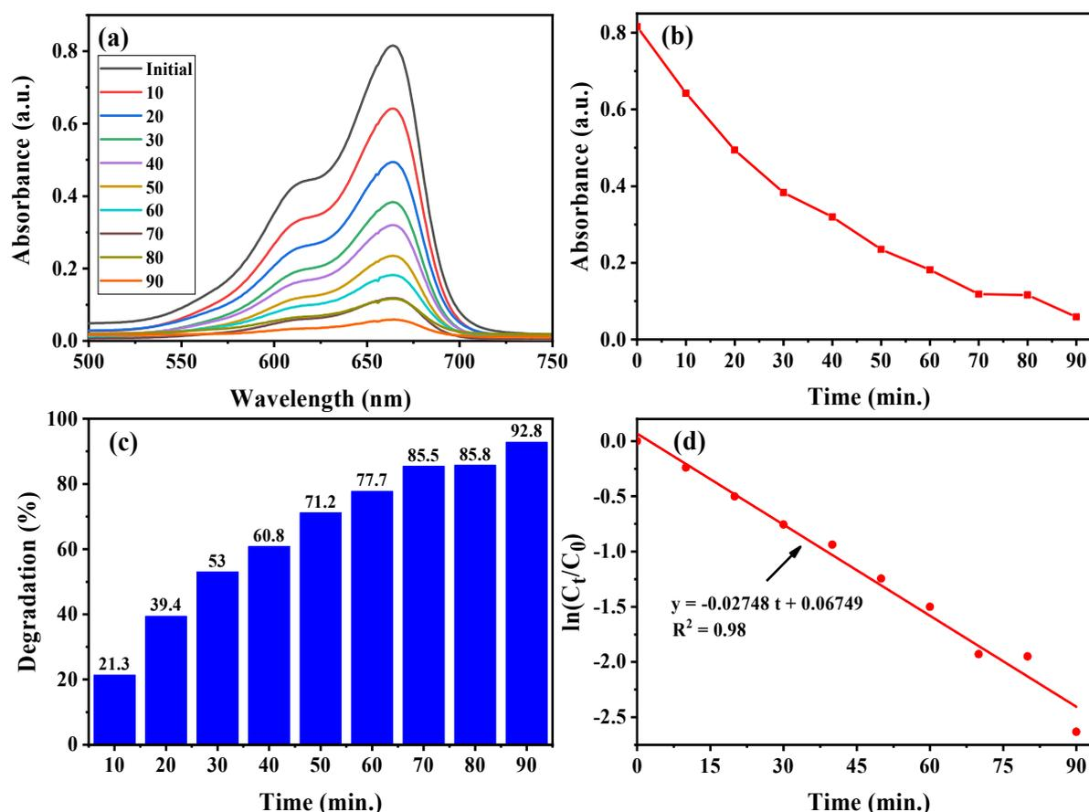
**Figure 7.** Change of absorbance with time (a,b), degradation achieved (c), and pseudo-first-order kinetics plot (d) for the degradation of MB under visible light for 90 min. using the synthesized rGO-CuO catalyst.
