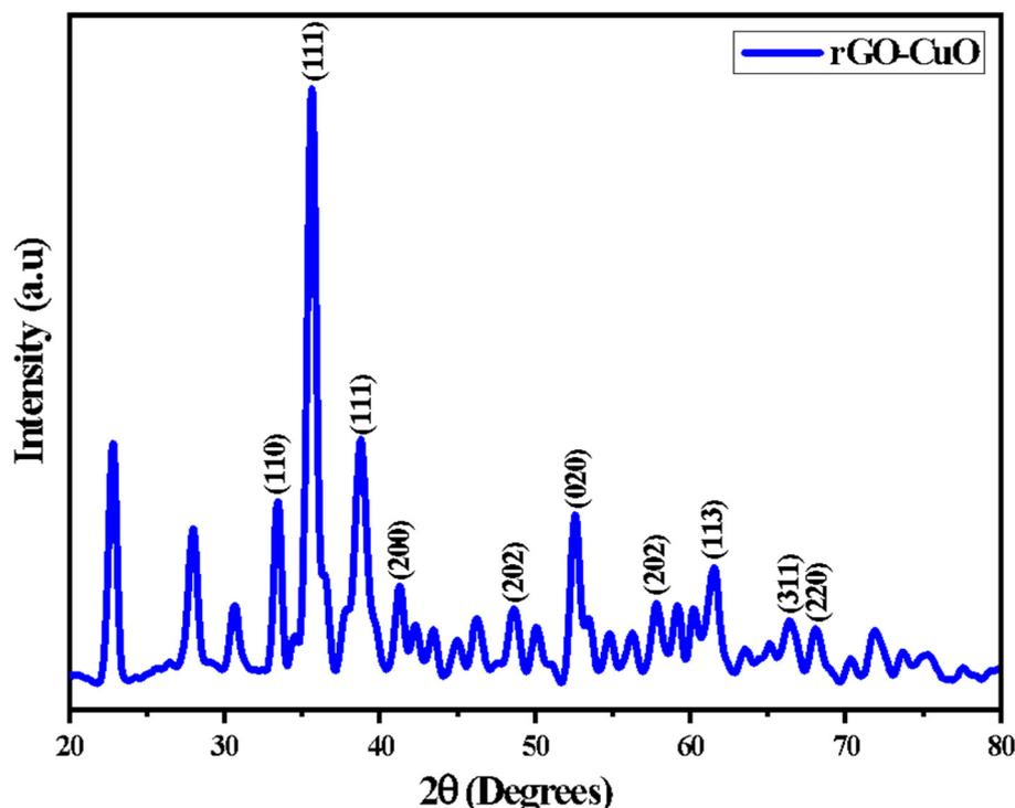
Figure 1. XRD pattern of as-synthesized rGO-CuO nanocomposites.
