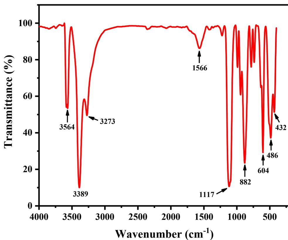
Figure 4. FTIR spectrum of the synthesized rGO-CuO nanocomposites.
