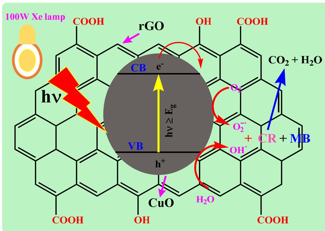
**Figure 8.** Formation of charge carriers and their transfer mechanism during the visible light assisted degradation of MB and CR dyes using rGO-CuO nanocomposites.
