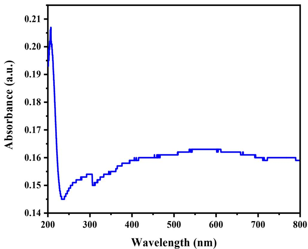
Figure 5. UV-vis absorption spectrum of rGO-CuO nanocomposites.
