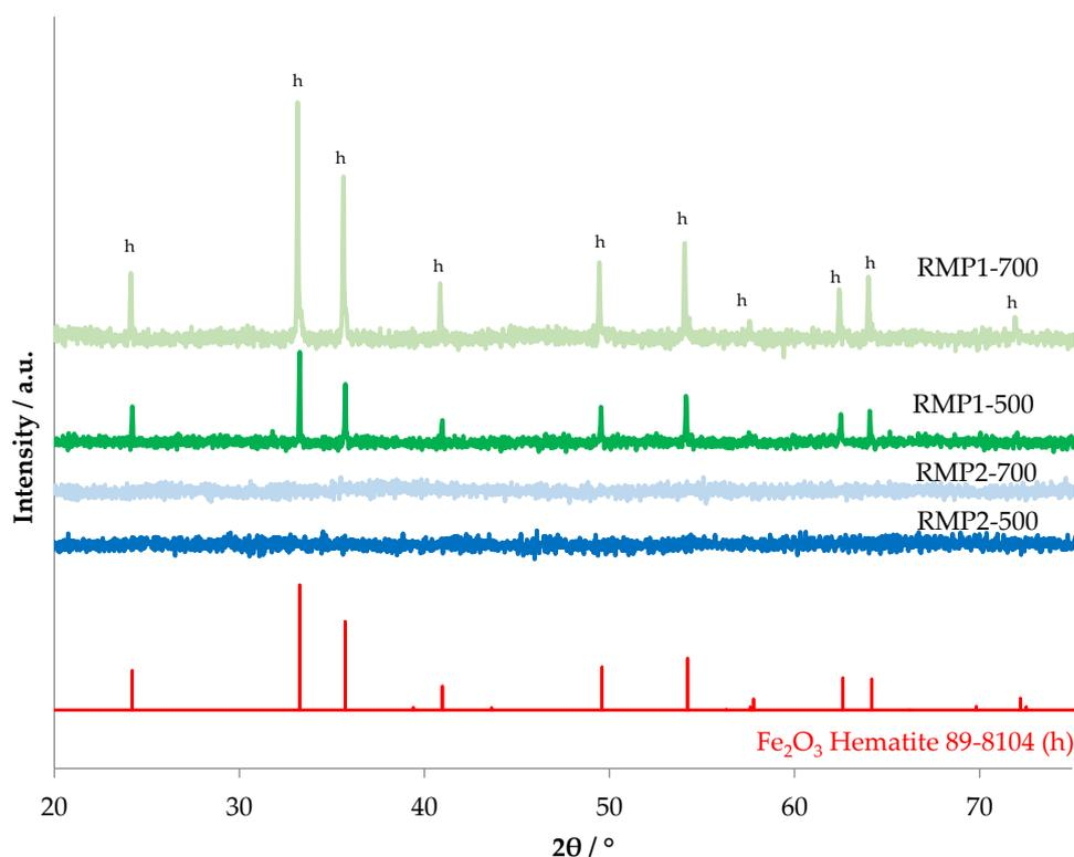
**Figure 8.** X-ray diffraction patterns of RMP samples calcined at 500 °C and 700 °C.
