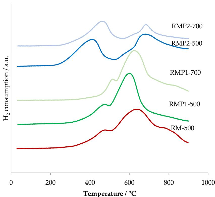
Figure 12. H<sub>2</sub>-TPR profiles of precipitated red mud samples calcined at 500 °C and 700 °C.
