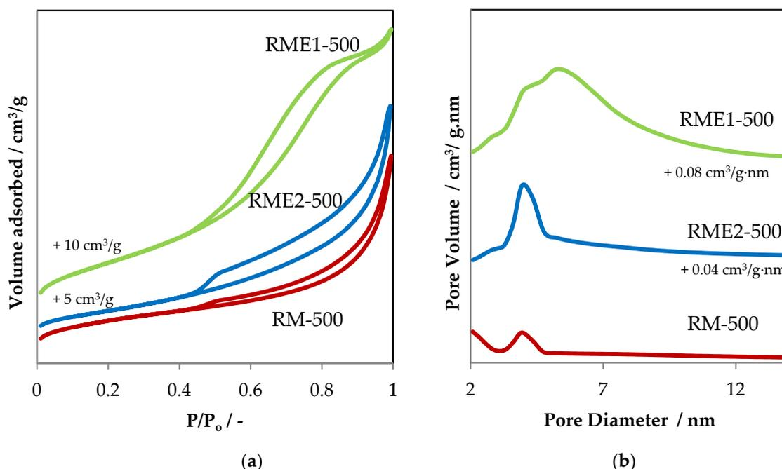
**Figure 1.** (a) N<sub>2</sub> adsorption–desorption isotherms and (b) the corresponding pore size distribution curves of RME and RM samples. The isotherms and the pore size distribution curves have been shifted by 5 and 10 cm<sup>3</sup>/g and 0.04 and 0.08 cm<sup>3</sup>/g.nm, respectively, for more clarity.
