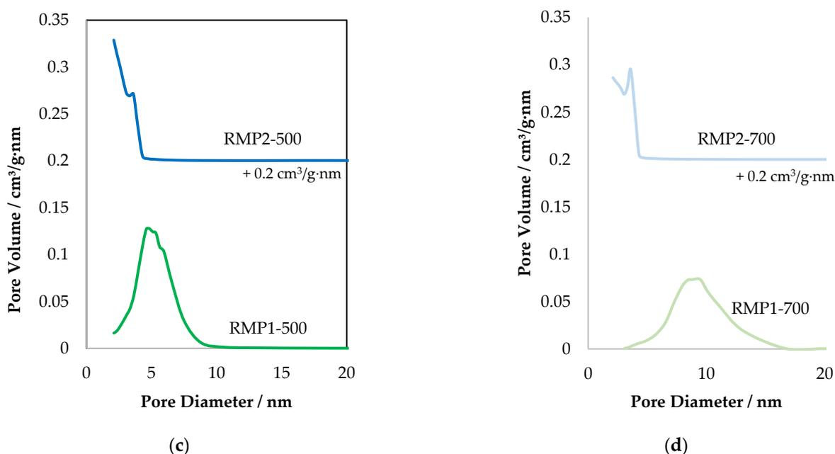
**Figure 7.** (a,b)  $N_2$  adsorption–desorption isotherms and (c,d) the corresponding pore size distribution curves of the RMP samples, shifted by  $0.2 \text{ cm}^3/\text{g}\cdot\text{nm}$ , for more clarity.
