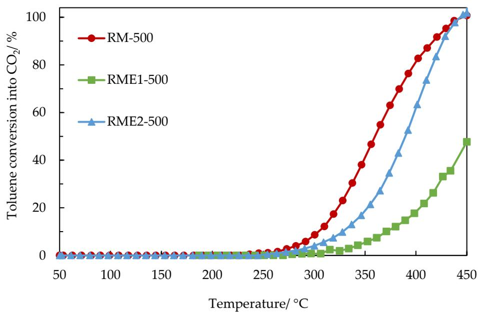
**Figure 6.** Toluene conversion to CO<sub>2</sub> as a function of the temperature in the presence of the unmodified calcined red mud (RM-500) and the evaporated catalysts (RME1-500 and RME2-500).
