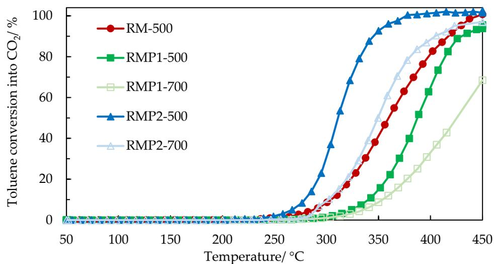
Figure 13. Toluene conversion to CO<sub>2</sub> as a function of the temperature in the presence of the calcined and precipitated catalysts (RM-500, RMP1-500, RMP2-500, RMP1-700, and RMP2-700).
