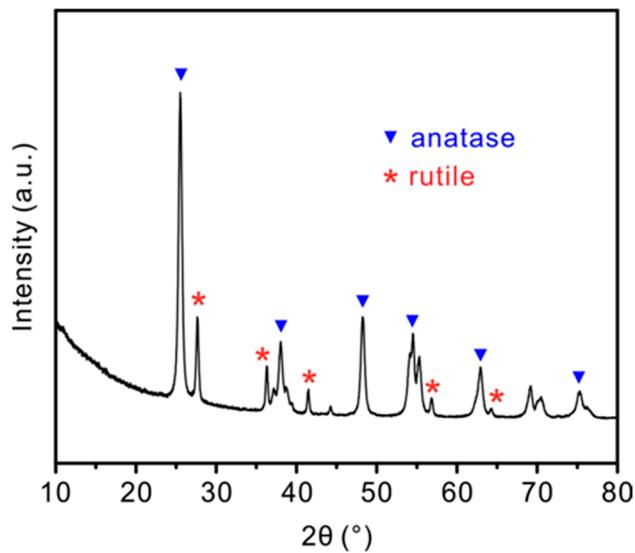
**Figure 1.** XRD pattern of the commercial P25 TiO<sub>2</sub> nanoparticles employed in the work.
