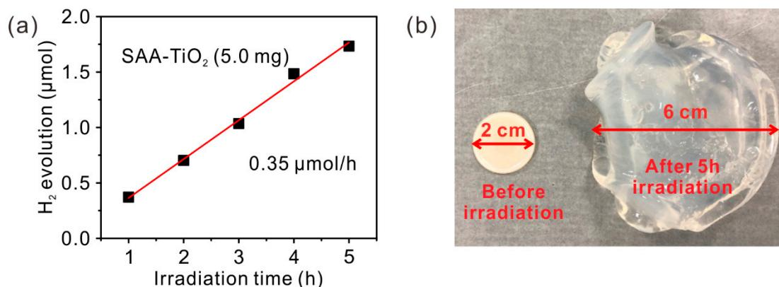
**Figure 6.** (a) Photocatalytic  $\text{H}_2$  evolution rates obtained by an SAA- $\text{TiO}_2$  sample with 5.0 mg added  $\text{TiO}_2$ . (b) Images of the SAA- $\text{TiO}_2$  sample before and after the reaction process involving 5 h of irradiation.
