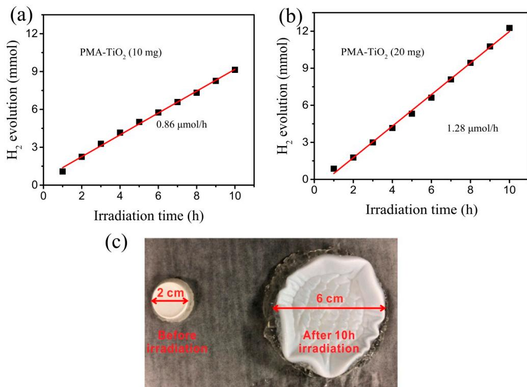
**Figure 5.** Photocatalytic H<sub>2</sub> evolution rates obtained with different concentrations of TiO<sub>2</sub> nanoparticles in the PMA hydrogel: (a) 10.0 mg; (b) 20.0 mg. (c) Images of a PMA-TiO<sub>2</sub> sample (20.0 mg TiO<sub>2</sub>) before and after reaction process involving 10 h of irradiation.
