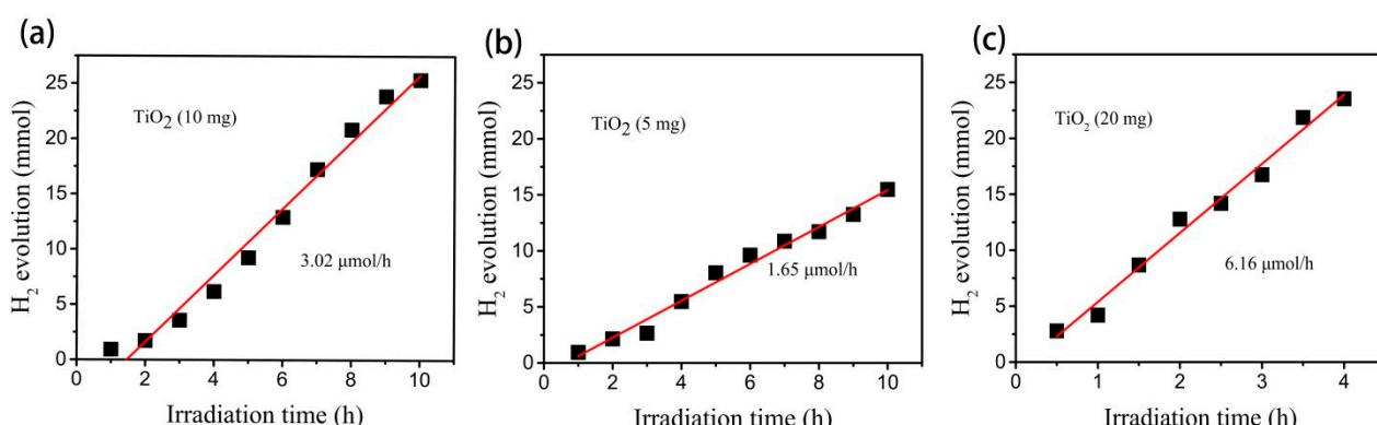
**Figure 4.** Photocatalytic H<sub>2</sub> evolution rates obtained with different concentrations of TiO<sub>2</sub> nanoparticle powder in deionized water with 10 mL triethanolamine (TEOA) added as the sacrificial reagent and a 300 W xenon lamp as a light source: (a) 5.0 mg; (b) 10.0 mg; (c) 20.0 mg.
