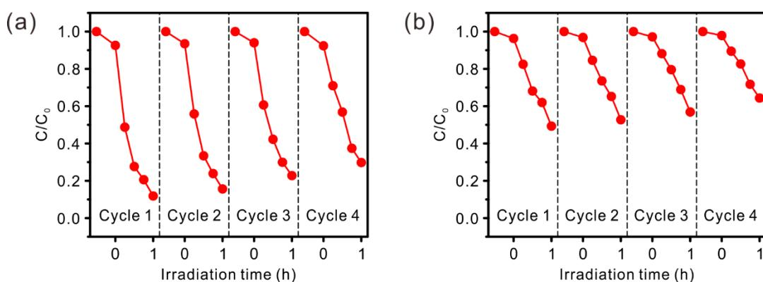
**Figure 8.** Cycling performance for the photodegradation of rhodamine B using (a) PMA-TiO<sub>2</sub> (20.0 mg) and (b) SAA-TiO<sub>2</sub> (5.0 mg).
