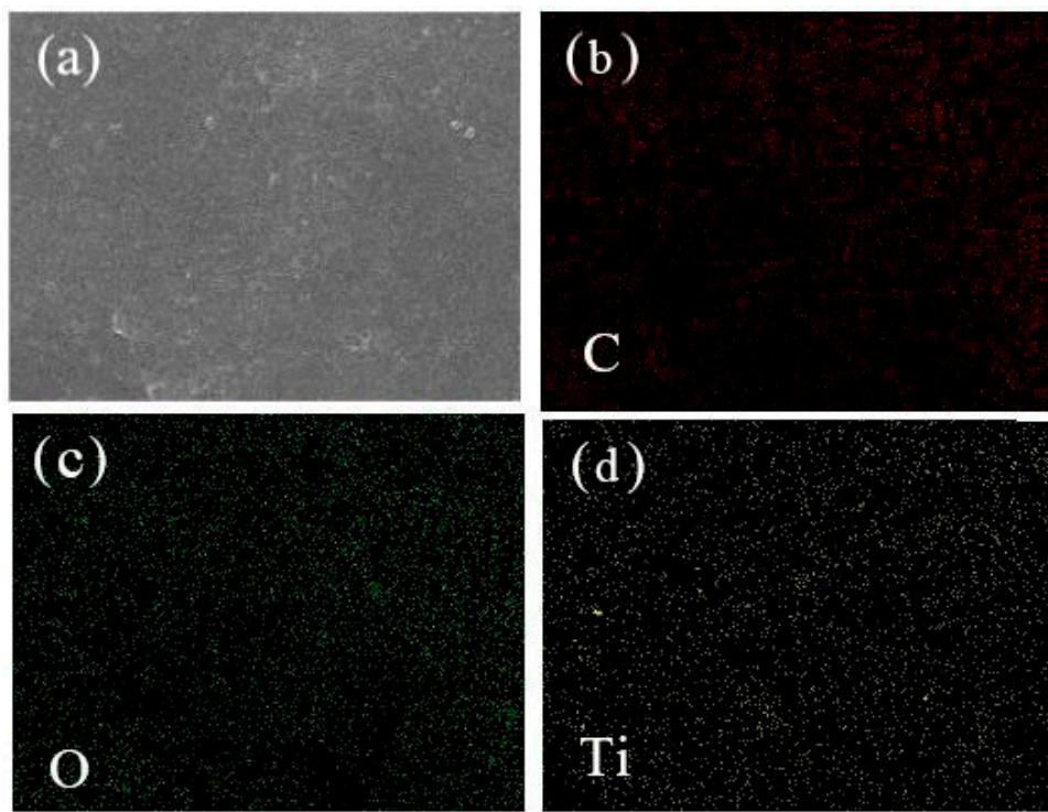
**Figure 2.** (a) SEM image of PMA- TiO<sub>2</sub> sample; (b) C, (c) O and (d) Ti EDS elemental mapping images of a representative PMA-TiO<sub>2</sub> hydrogel sample.
