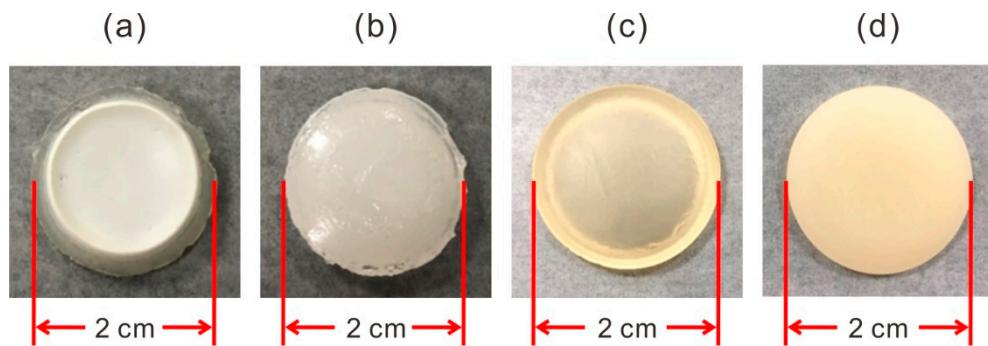
**Figure 3.** Images of standard hydrogel samples: (a) bottom side of a PMA-TiO<sub>2</sub> sample (20.0 mg added TiO<sub>2</sub>) with a thin layer of TiO<sub>2</sub> nanoparticles near the surface; (b) top side of the PMA-TiO<sub>2</sub> sample with a transparent surface; (c) bottom side of an SAA hydrogel sample (5.0 mg added TiO<sub>2</sub>) with a transparent surface; (d) top side the SAA-TiO<sub>2</sub> sample with a uniform distribution of TiO<sub>2</sub> nanoparticles.
