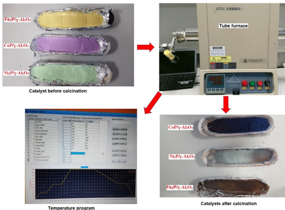
Figure 1. Calcination of \text{Ni}_2\text{P}/\gamma\text{-Al}_2\text{O}_3 , \text{CoP}/\gamma\text{-Al}_2\text{O}_3 , and \text{Fe}_2\text{P}/\gamma\text{-Al}_2\text{O}_3 supported catalysts.
