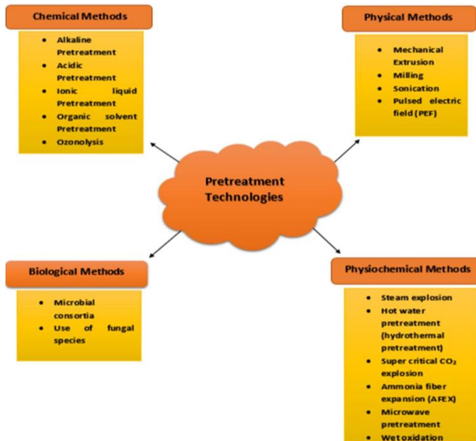
**Figure 4.** Flowchart of different pretreatment technologies.
