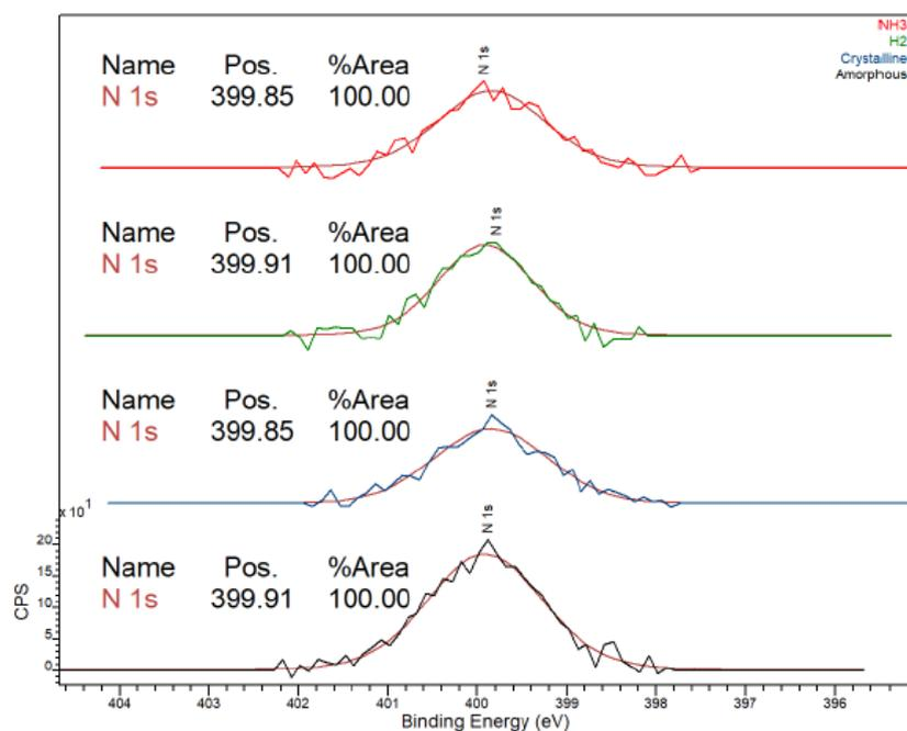
Figure S5: XPS spectra of N 1s of A-TiO<sub>2</sub> (black), C-TiO<sub>2</sub> (blue), H-TiO<sub>2</sub> (green) and N-TiO<sub>2</sub> (red).
