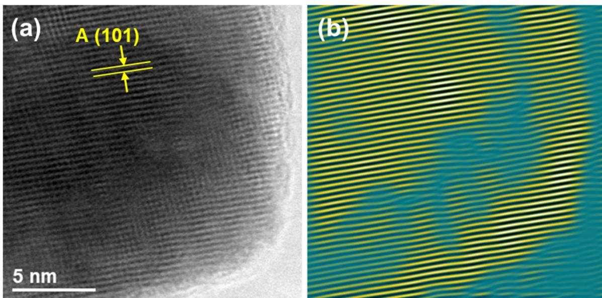
Figure S3: High-resolution ABF-STEM image of anatase nanoparticle N-TiO<sub>2</sub> (a) and the corresponding filtered image using  $g_{101}$  (b). Areas of nano-scale lattice distortion were detected, attributed to accumulation of point defects.
