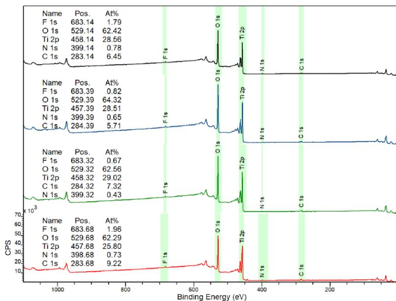
Figure S4: Survey XPS spectra of A-TiO<sub>2</sub> (black), C-TiO<sub>2</sub> (blue), H-TiO<sub>2</sub> (green) and N-TiO<sub>2</sub> (red). Atomic percentages are given on the graph.
