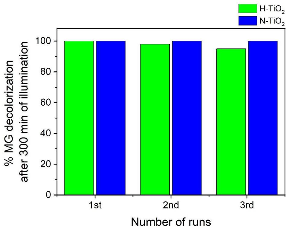
Figure S6: Recycling experiments of the H-TiO<sub>2</sub> and N-TiO<sub>2</sub> samples for three consecutive cycles of 300 min each. In each round a fresh solution of 5 mg L<sup>-1</sup> MG was photocatalytically treated by 0.5 g L<sup>-1</sup> of recovered photocatalyst under visible light illumination.
