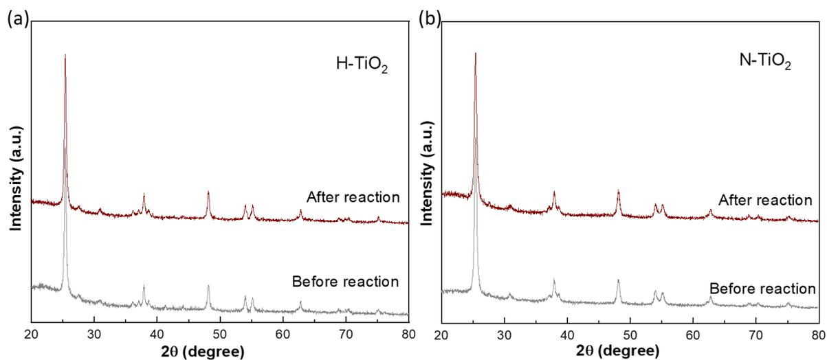
Figure S7: XRD patterns of the H-TiO<sub>2</sub> (a) and N-TiO<sub>2</sub> (b) samples before and after the recycling experiments of Fig. S6.
