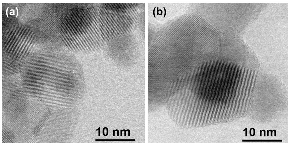
Figure S1: ABF-STEM images of the same magnification from C-TiO<sub>2</sub> (a) and N-TiO<sub>2</sub> (b). Annealing in NH<sub>3</sub> atmosphere resulted in larger grains reaching a maximum size ~25 nm, while the maximum grain size observed after annealing in air was ~15 nm.
