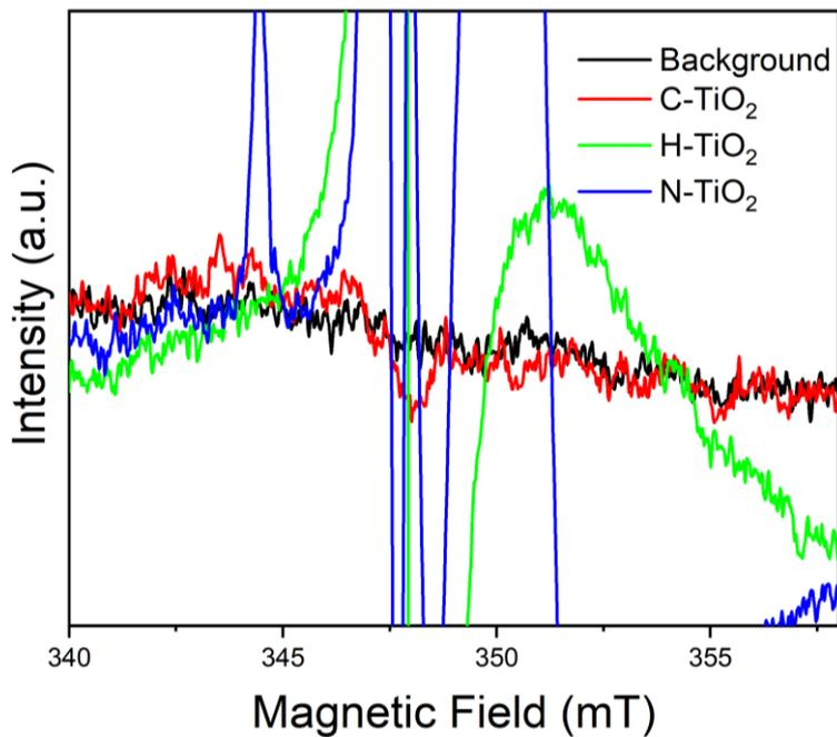
Figure S2: A higher magnification of the EPR spectra of paramagnetic species in C-TiO<sub>2</sub>, H-TiO<sub>2</sub> and N-TiO<sub>2</sub>.
