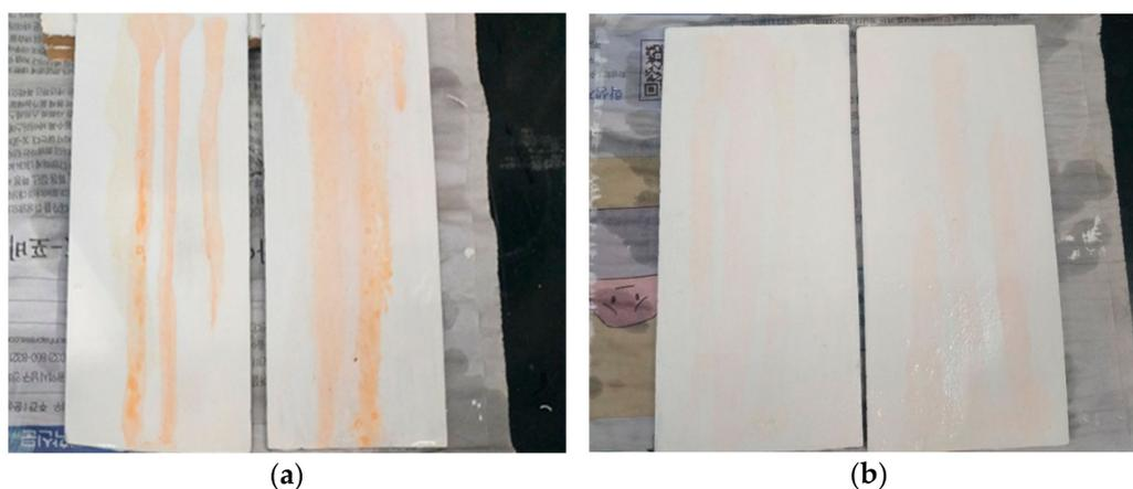
**Figure 8.** Images of general paint coating (a), and INCN-20 coating (b) after oil spraying followed by washing.
