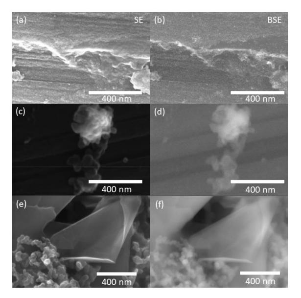
**Figure S1.** Scanning electron microscopy images of the surfaces of the ALD-prepared electrodes. The images in the left column were generated made by the secondary electron (SE) technique and the images on the right by the backscattered electron (BSE) technique. (**a**,**b**) 20c Pt; (**c**,**d**) 25c TiO2 + 20c Pt; (**e**,**f**) bare carbon paper.
