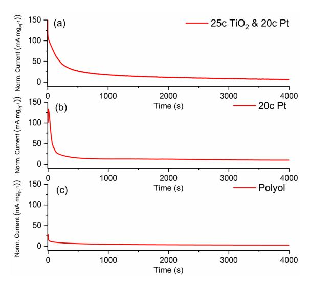
**Figure S4.** Chronoamperometric measurements of the ALD-prepared catalysts: 25c TiO2 + 20c Pt (**a**); 20c Pt (**b**); Polyol catalyst (**c**).
