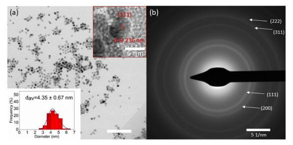
Figure S3. Transmission electron microscopic image (a) and electron diffractogram (b) of the polyol catalyst.
