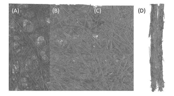
**Figure S2.** Micro-CT images of the bare AvCarb P75 carbon paper (**A**), the 20c Pt electrode (**B**), the 25c TiO2 + 20c Pt electrode (**C**), and side view of the 20c Pt electrode (**D**).
