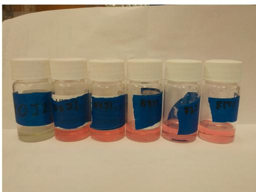
**Figure A3.** Photograph of 90% w/w HAN + water samples no additive, 0.05%, 0.1%, 0.5%, 1%, and 5% Bipy respectively, from left to right.
