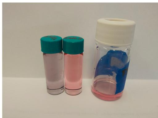
**Figure A4.** Photograph of samples with 7.5 mole ratio of Bipy:Cu and Bipy:Fe compared with 1% Bipy all in 90% HAN solution.
