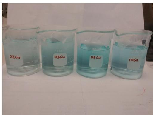
**Figure A1.** Photograph of samples with 100 ppm Cu with 2, 3, 5, and 10 times as many moles of Bipy added respectively, from left to right in  $\text{HNO}_3$  solution.
